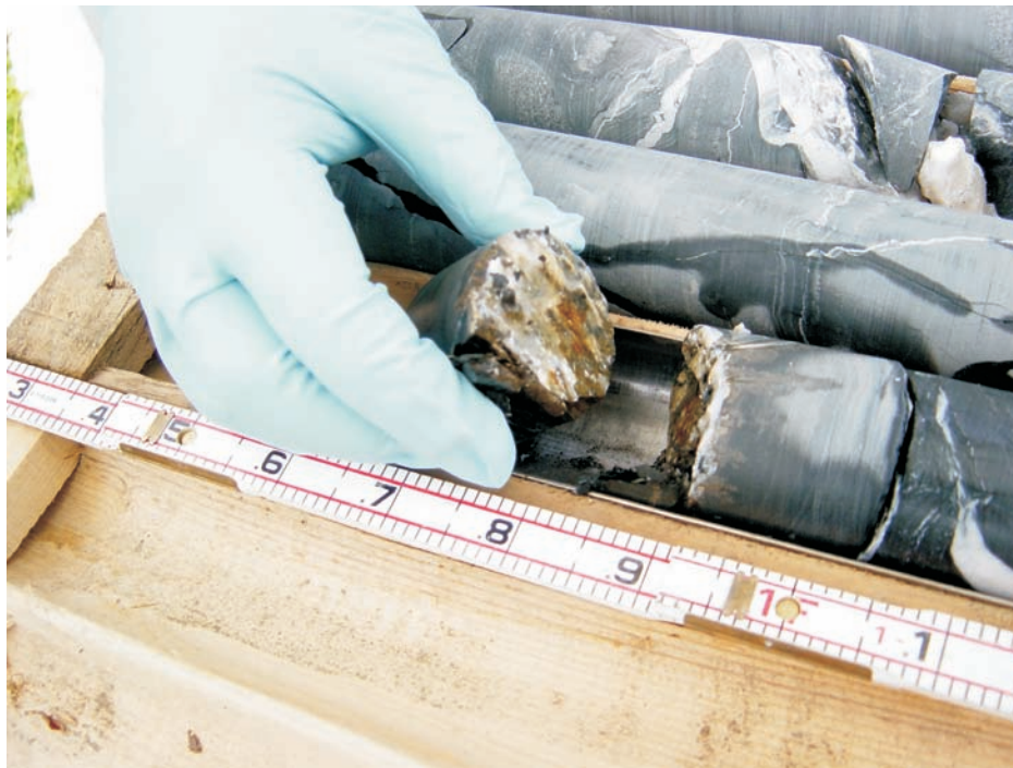
Figure 7.1.4-1. Fracture at 23.4 meters (76.9 feet) bgs in BD I-5-6.
