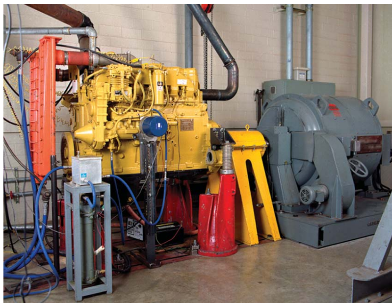
Diesel engine in a dynamometer test cell at Southwest Research Institute
