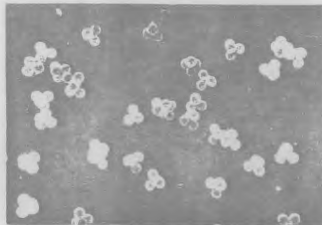
(c) Micrograph of tetrahedral aggregates of four latex spheres of 7.9 \times 10^{-5} cm diameter (Stereoscan scanning electron microscope)
