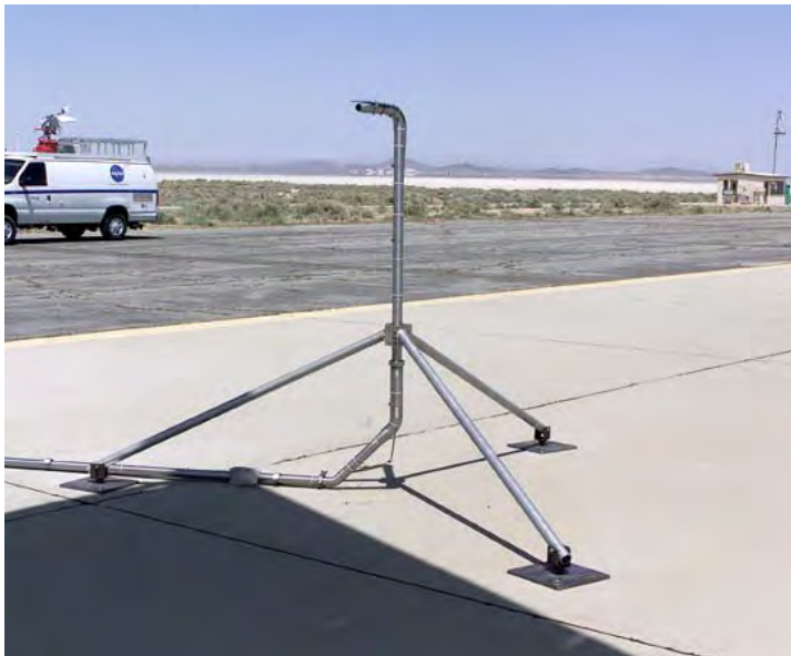
Figure 2-2. DEAL 30-m exhaust plume probe assembly for APEX-1.
