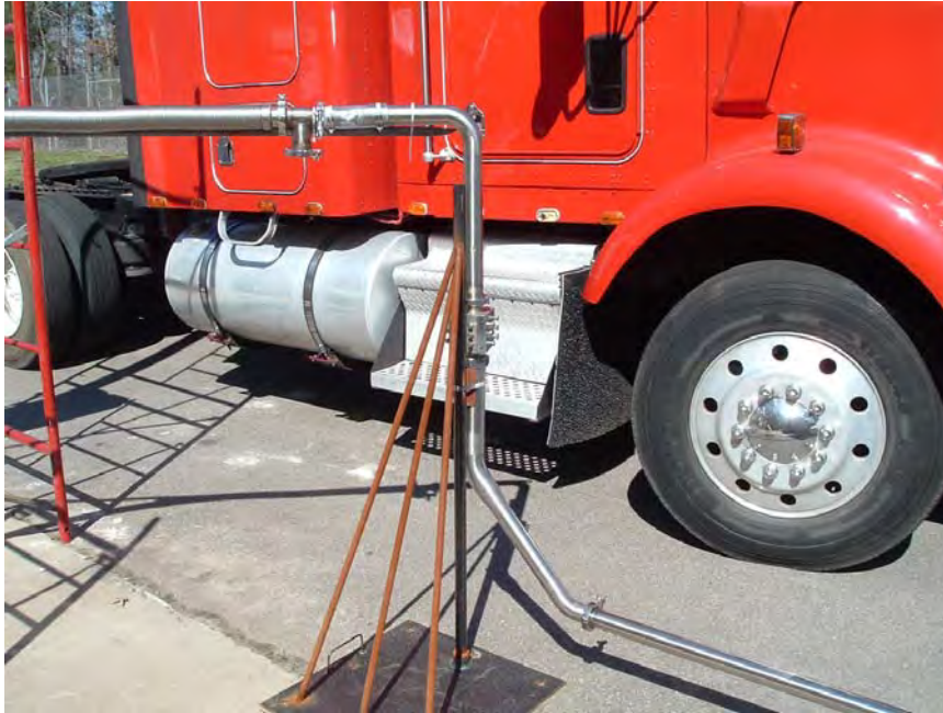
Figure 4-2. Line loss sample location at probe inlet.
