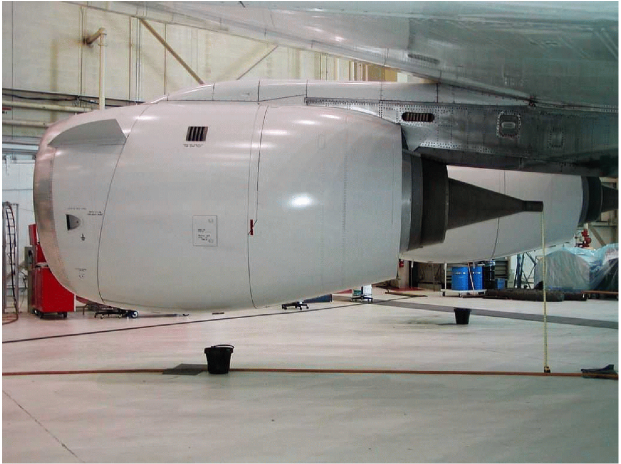
Figure 2-9. CFMI Model CFM56-2C1 jet engine tested during APEX-1.
