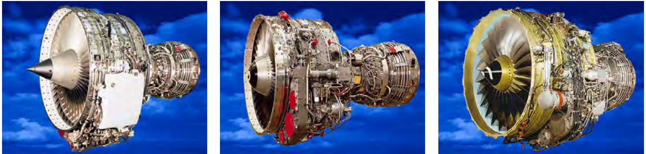
Figure 2-10. CFMI Model CFM56 engines: CFM56-2 (left), CFM56-3 (center), and CFM56-7 (right).
