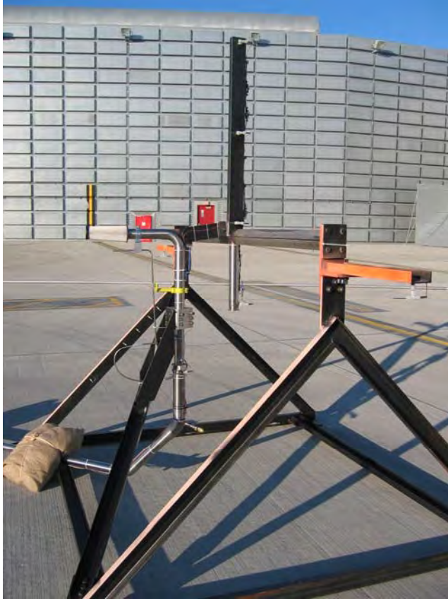
Figure 2-5. DEAL 30-meter exhaust plume probe assembly for APEX-2.
