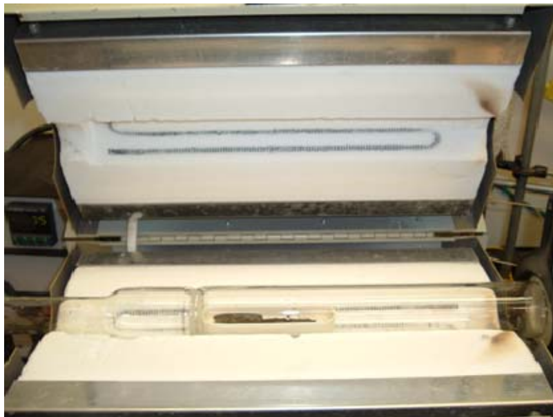
Figure 2-2. Asphalt and wallboard simulation quartz reactor and furnace with sample
