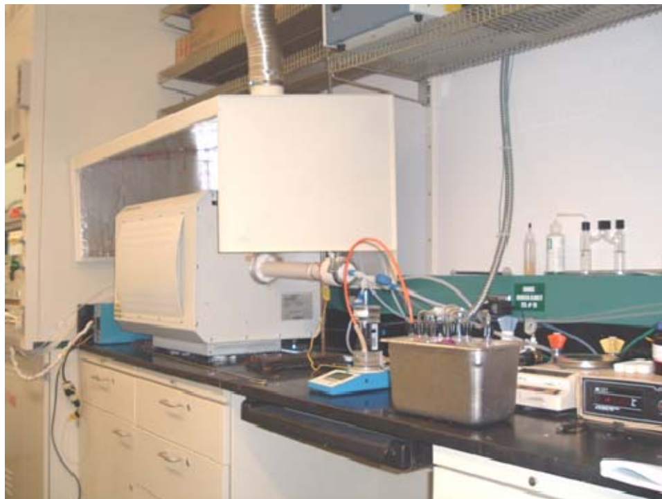
Figure 2-3. High temperature cement simulation furnace with Method 29 mini-impinger train
