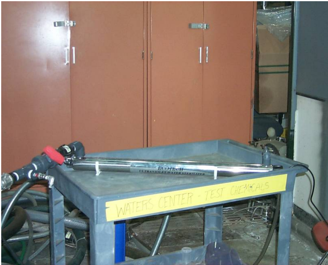
Figure 2-9. UV System at T&E Facility
