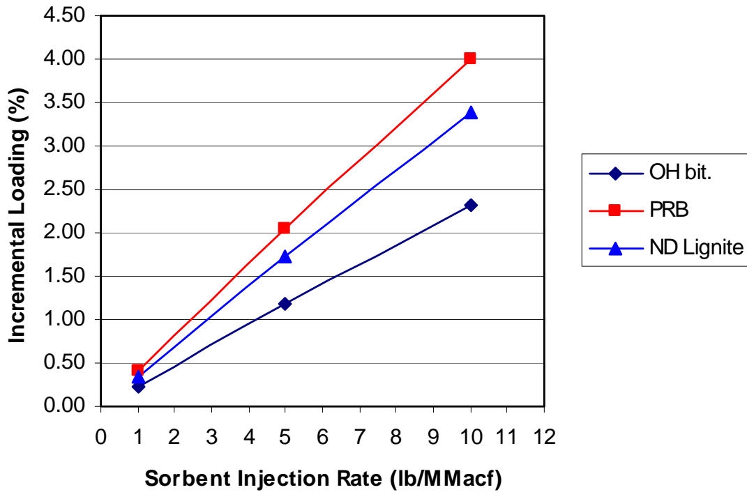
Figure 17. Calculated incremental particulate loading in the flue gas from sorbent injection
