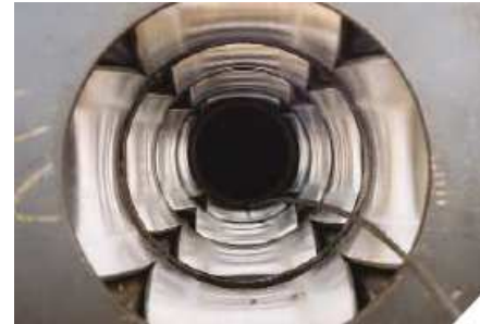
Figure 3-11. Roller Reduction Unit for PolyFlex
