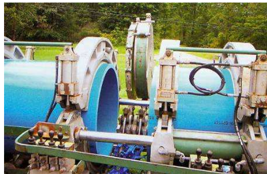
Figure 3-22. Fusion of PVC Joint
