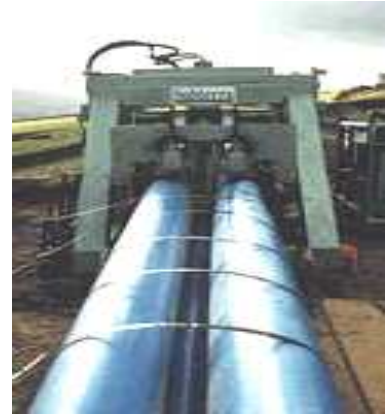
Figure 3-15. Subline Forming into “C” Shape
