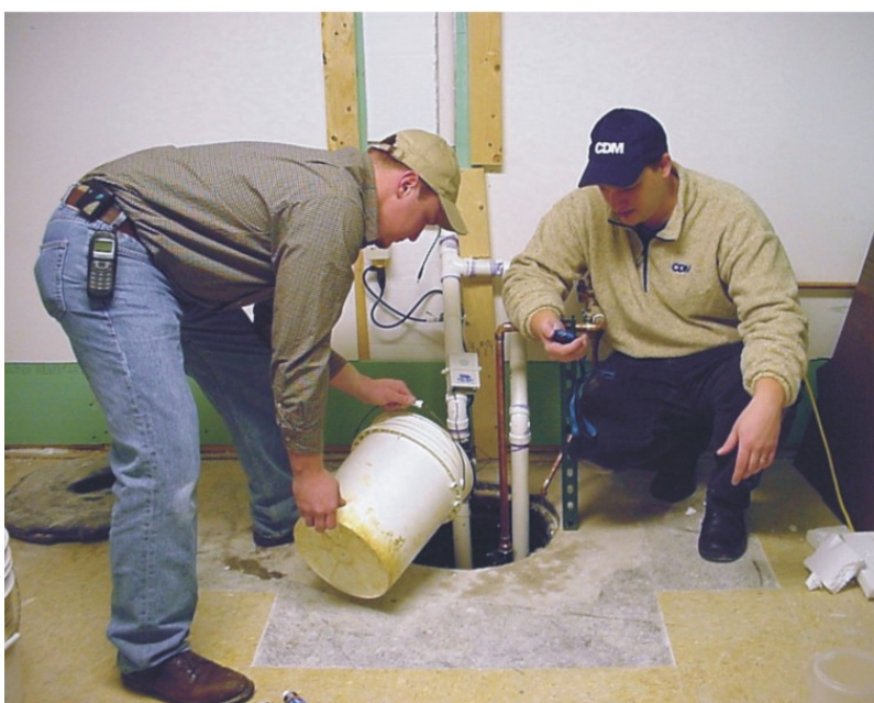
Figure 8-6. Testing pumping rate to support monitoring of a disconnected footing drain.
