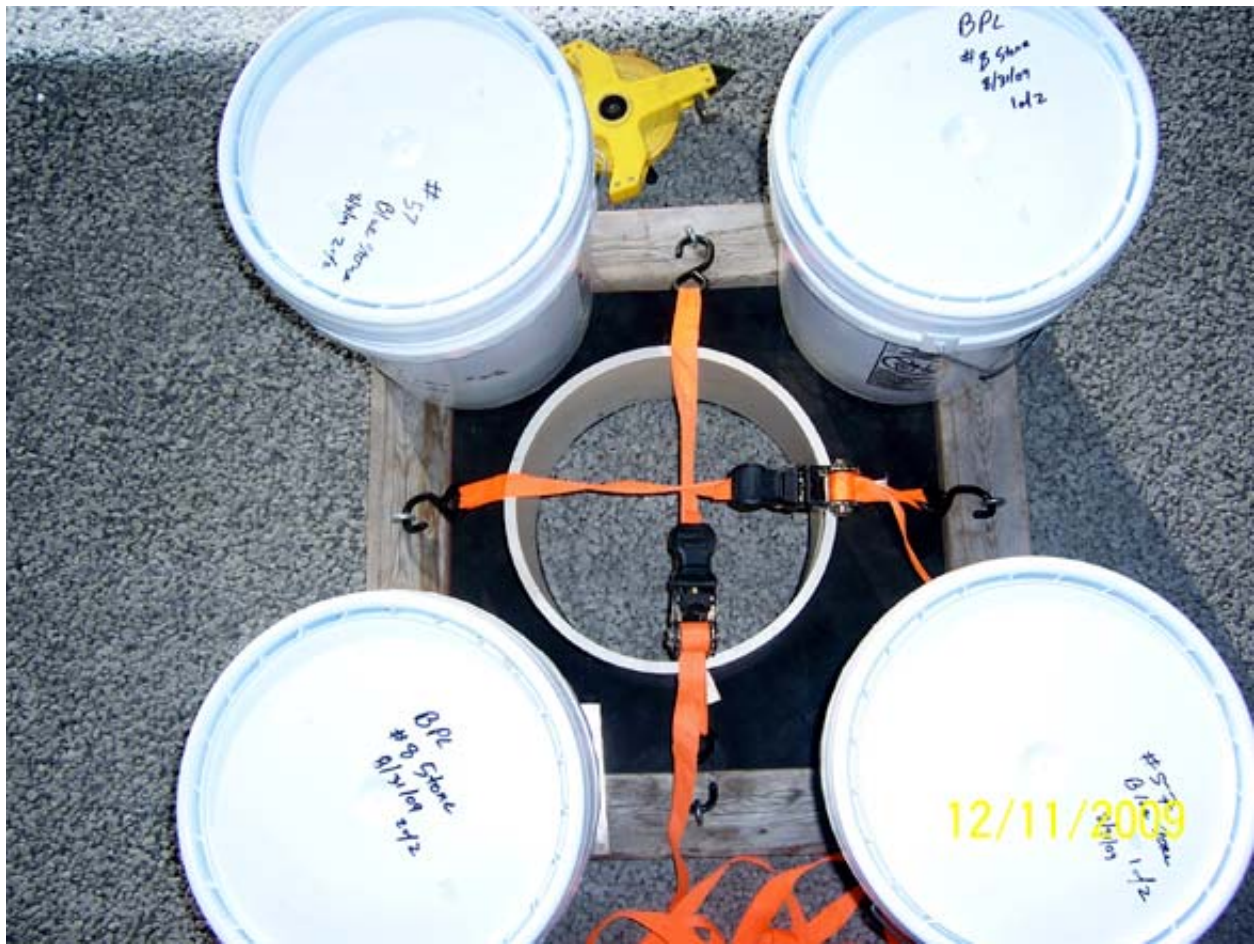
Figure 1. The weight of the 5-gallon buckets of stone applied to the PVC compresses the Neoprene sheeting to form a leak-free seal with the parking surface. Collectively the buckets weigh 150 to 200 kg.
