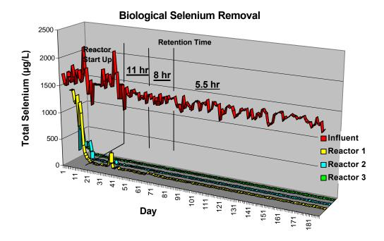
Figure 2-4. BSeR<sup>™</sup> process pilot-scale reactor summary graph.
