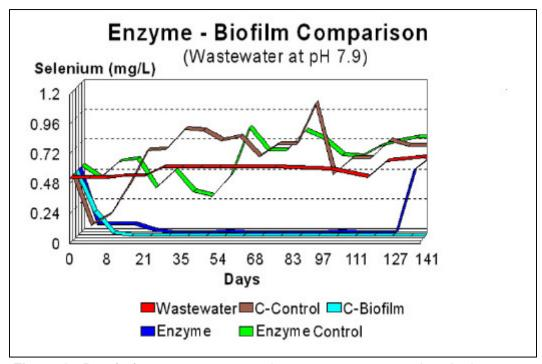
**Figure 8**. Proof-of concept reactor testing compares enzymatic selenium reduction to live microbial systems.
