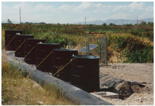
Figure 1-7. Field-scale BSeR™ process reactor.
