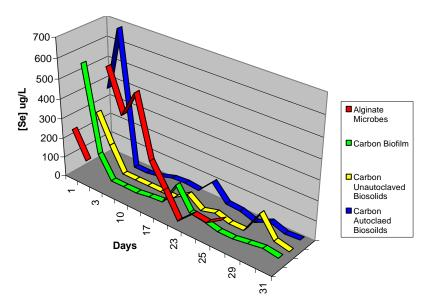
Figure D-11. Laboratory Bioreactor Series 2. The second series of carbon, carbon-biosolids, and alginate columns used to measure selenium reduction using KUCC waters (-2 mg/L). Columns used a 12-hr retention time and were run at ambient temperature under anaerobic conditions. The alginate column was used to measure relative effectiveness of various different selenium reducing microbes.
