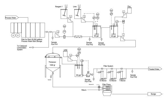
Figure 1-2. Ferrihydrite precipitation process flow diagram.
