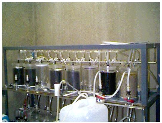
Figure D-13. Second series of BSeR<sup>™</sup> laboratory reactors.
