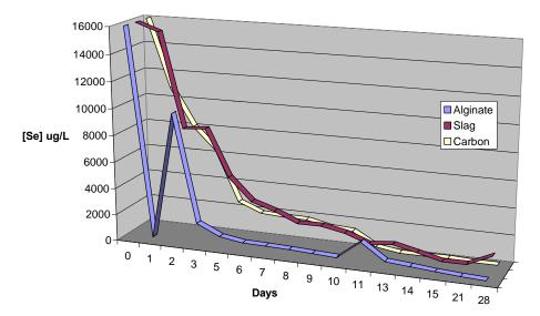
Figure D-10. Laboratory Bioreactor Series 1. The initial carbon, slag, and alginate columns that were used to measure selenium reduction using KUCC waters (-14.7 mg/L). Columns used a 24-hr retention time until day 10 when they were switched to a 12-hr retention time. Columns were run at ambient temperature under anaerobic conditions. The alginate column was used to measure relative effectiveness of various different selenium reducing microbes.
