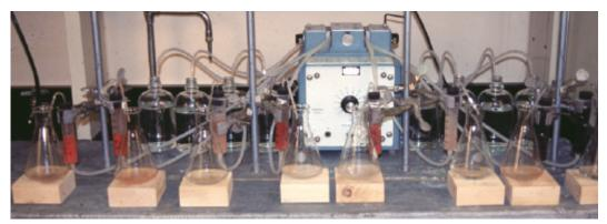
Figure 5. Bench scale reactor test apparatus.
