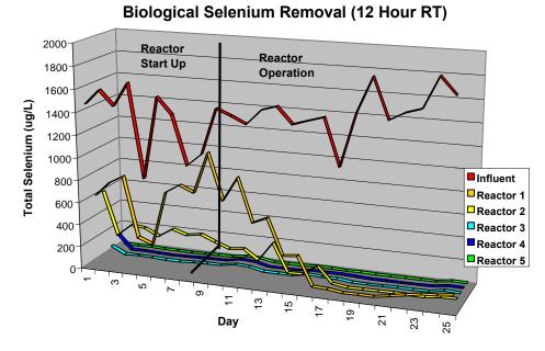
Figure 2-3. Series 1 Pilot-scale BSeR<sup>™</sup> process operation at a 12-hr retention time per reactor.
