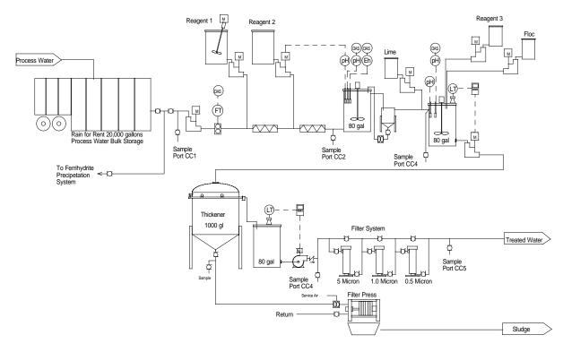
Figure 1-4. Catalyzed cementation process flow diagram.
