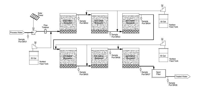
Figure 1-6. BSeR<sup>™</sup> process flow diagram.
