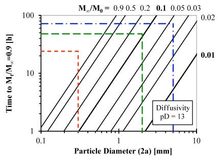
Figure 2. Contact time required for a species with an observed diffusivity of  $10^{-13}$  m<sup>2</sup>/s to reach 90% of equilibrium ( $M_{\tau}/M_{\odot} = 0.9$ ) based on mass transport as functions of particle diameter and fractional solubility ( $M_{\infty}/M_{\odot}$ ). Figure modified from Garrabrants, 1997.
