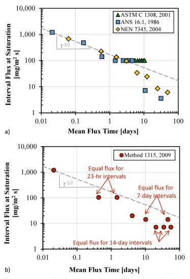
Figure 5. Hypothetical internal mass flux assuming the exchange intervals in the tank leach test were long enough to results in equilibrium between solid and bulk liquid phases: (a) common test methods and (b) *Method 1315*.
