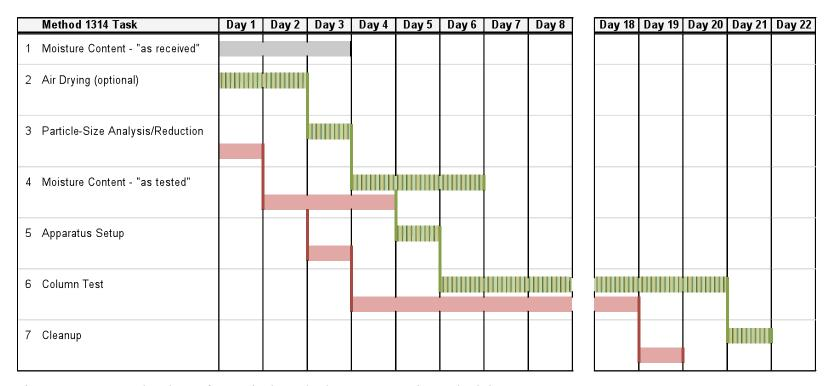
Figure 9. Gantt Style Chart of a Typical Method 1314 Processing Schedule.
