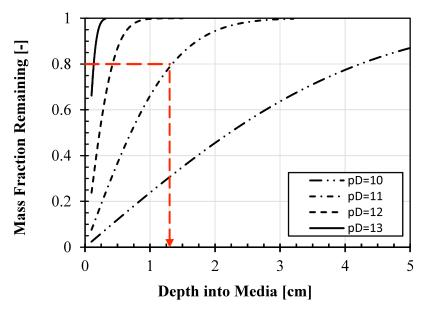
Figure 4. Evaluation of depth of depletion  $C(x,t)/C_0=0.8$  as a function of diffusion coefficient (pD is the negative logarithm of the diffusion coefficient).
