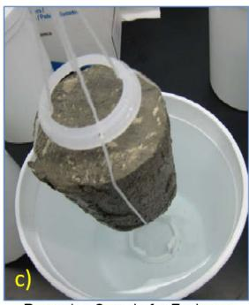
Removing Sample for Exchange
