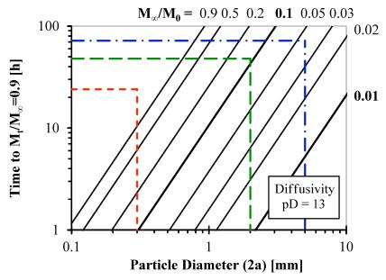
Figure 6. Contact time required for a species with an observed diffusivity of  $10^{-13}$  m<sup>2</sup>/s to reach 90% of equilibrium ( $M_t/M_{\odot} = 0.9$ ) based on mass transport as functions of particle diameter and fractional solubility ( $M_{\odot}/M_0$ ). Figure modified from Garrabrants, 1997.
