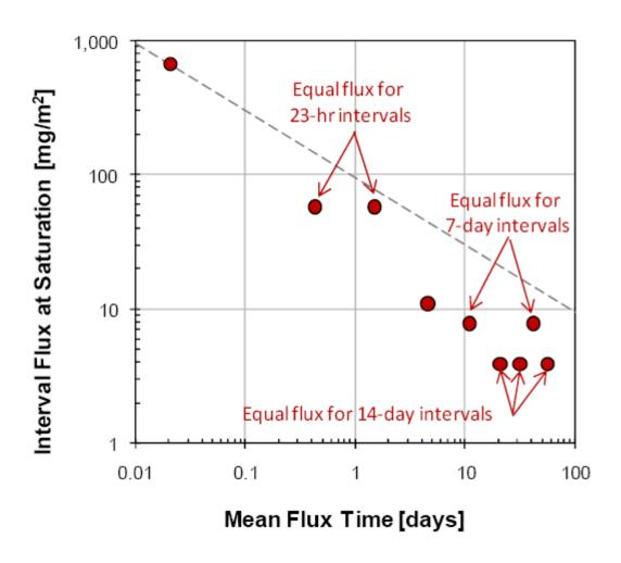
NOTE: This figure assumes that the concentration in the eluate approaches saturation during the leaching interval (i.e., the driving force for diffusion approaches zero). When the leaching solution is saturated, the resulting mass release and interval flux is constant for intervals of the same duration.
