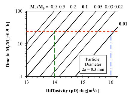
Figure 7. Contact time required for a particle of 0.3 mm diameter to reach 90% of equilibrium ( $M_t/M_{\odot} = 0.9$ ) as function of diffusivity and fractional solubility ( $M_{\odot}/M_0$ ). Figure modified from Garrabrants, 1997.
