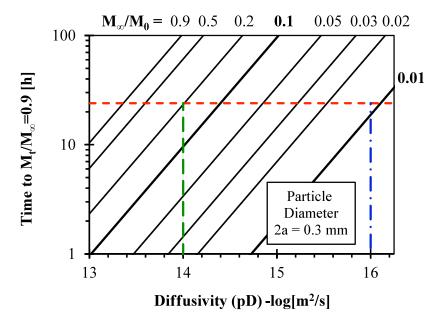
Figure 3. Contact time required for a particle of 0.3 mm diameter to reach 90% of equilibrium ( $M_t/M_{\odot} = 0.9$ ) as function of diffusivity and fractional solubility ( $M_{\odot}/M_0$ ). Figure modified from Garrabrants, 1997.
