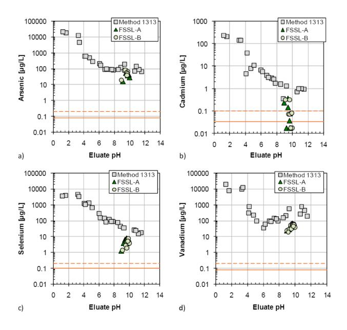
NOTE: Orange lines represent cumulative release if all eluate extracts were at the quantitation limit (dashed) and detection limit (solid). Chemical analyses below the detection limit are shown at ½ the detection limit value.
