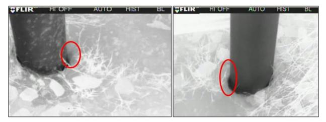
Figure 3-7. Screenshots from FLIR Camera of Fugitive Leaks from Base of Gas Wells at Site A.
