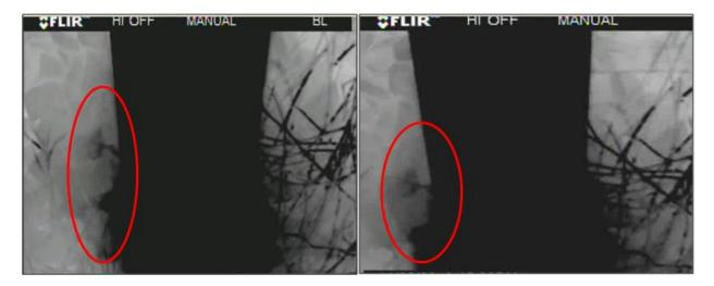
Figure 3-8. Additional Screenshots from FLIR Camera of Fugitive Leaks from Base of Gas Wells at Site A.
