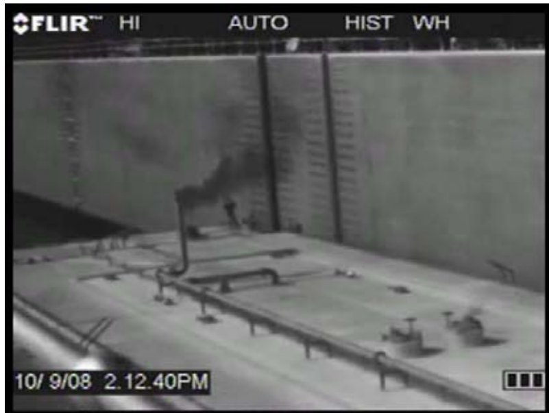
Figure 3-19. Example #2 from Ground Survey with LDEQ Camera – Leaking Vent from Barge L23- Total OTM 10 Mass Emission from Barge 0.490 g/s
