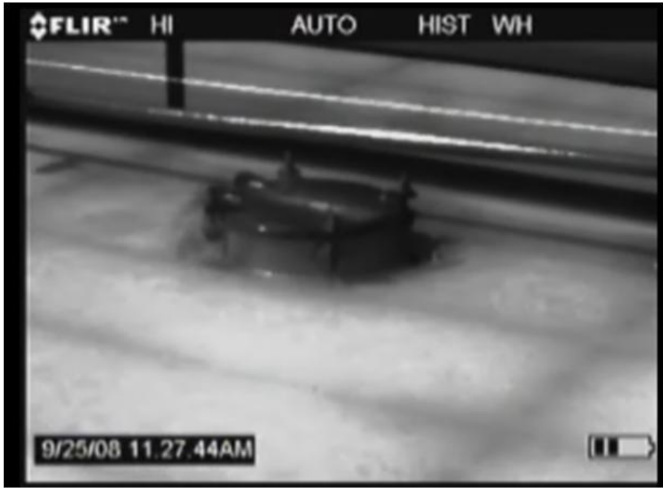
Figure D-8. Leak from Barge G2 (captured while onboard barge)
