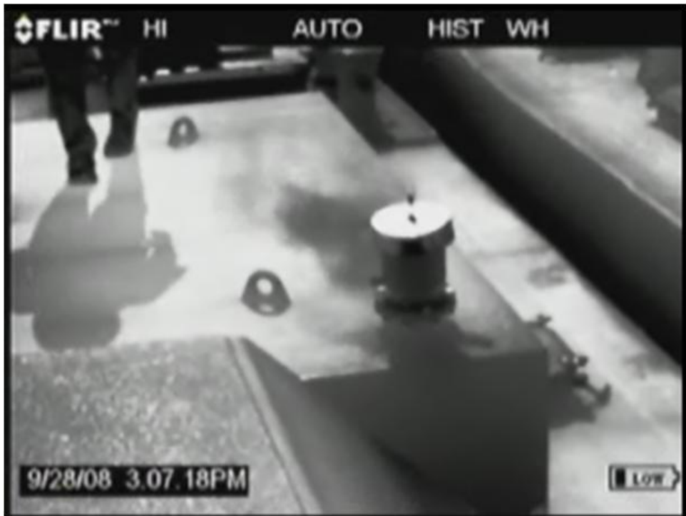
Figure D-37. Leak from Barge G8 (captured while onboard barge)
