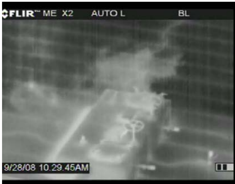
Figure 3-18. Example #1 from Ground Survey with LDEQ Camera – Leaking Hatch from Barge L10 (there was no OTM 10 emission flux measurement for this time period)
