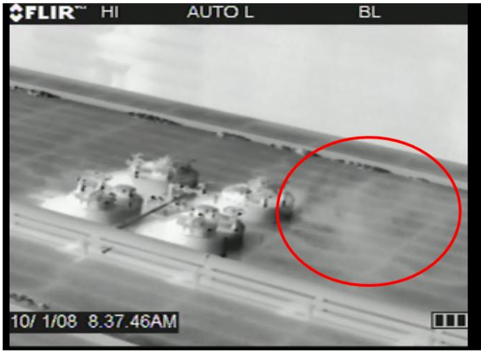
Figure E-3. Leak from Hatch 10/1
