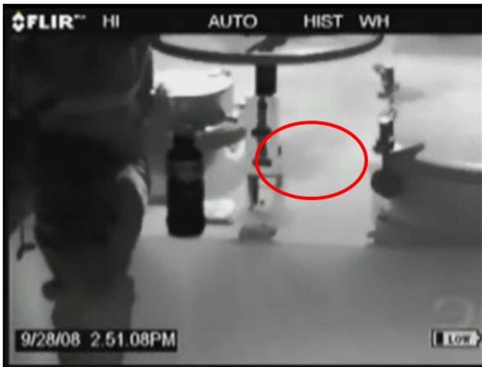
Figure D-32. Leak from Barge G8 (captured while onboard barge)
