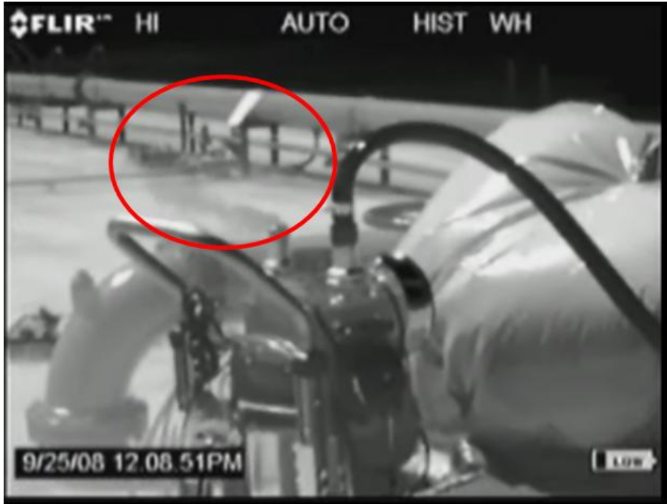
Figure D-12. Leak from Barge G3 (captured while onboard barge)
