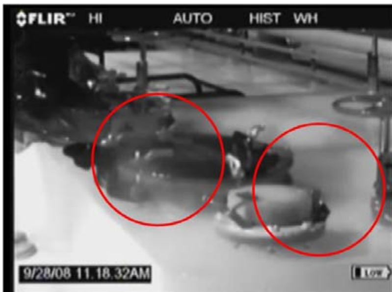
Figure 3-13. Leak from Cargo Hatch on Barge G7- Mass Leak 3.12 g/s
