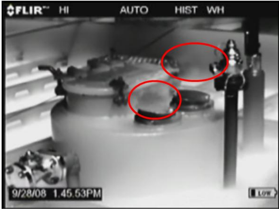
Figure D-29. Leak from Barge G8 (captured while onboard barge)
