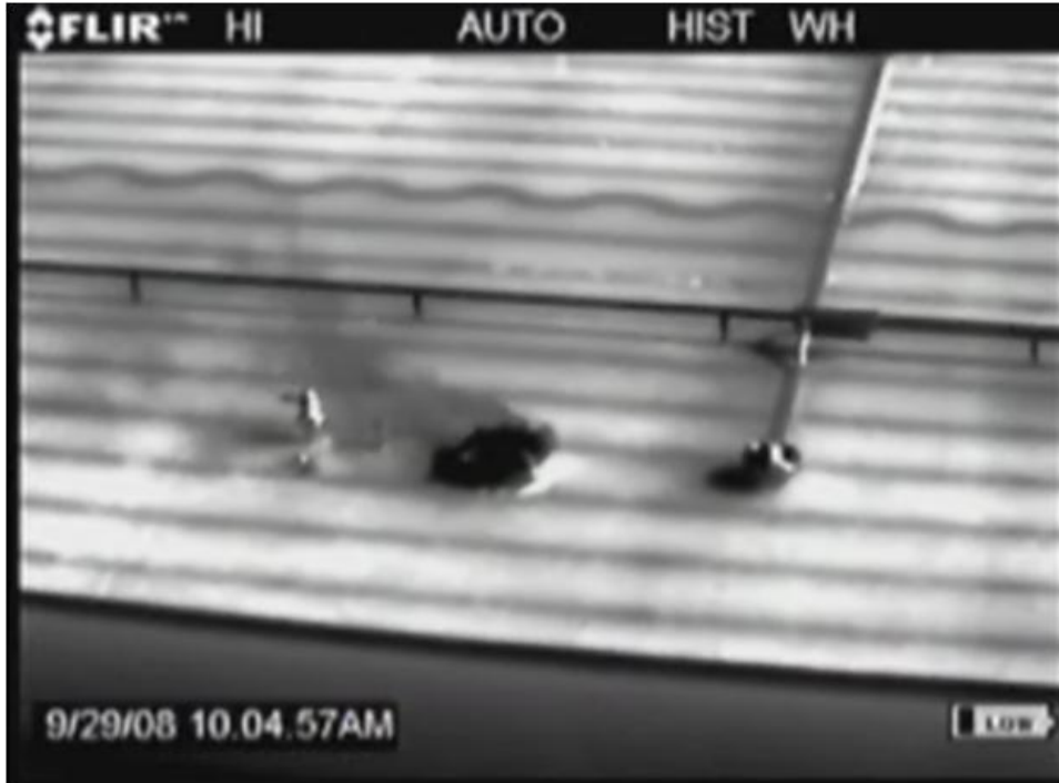
Figure D-40. Leak from Barge L6 (captured while barge in lock)
