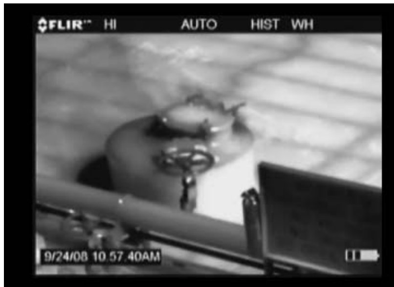
Figure 3-15. Example #1 from LSI Ground Survey – Leaking Hatch on Barge L1- Total Mass Emission from Barge 0.521 g/s
