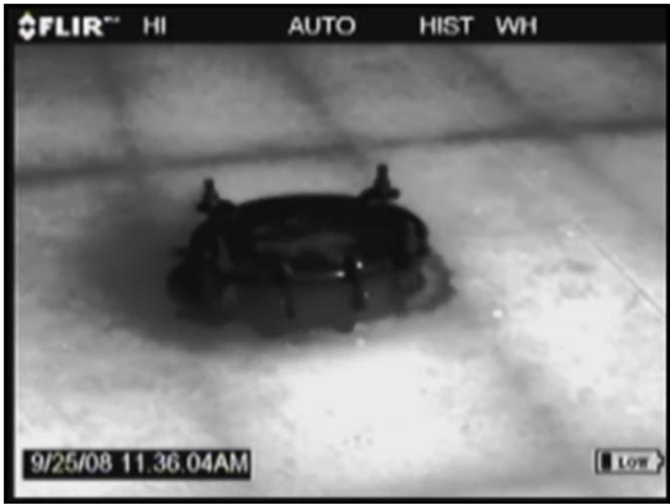
Figure D-11. Leak from Barge G2 (captured while onboard barge)
