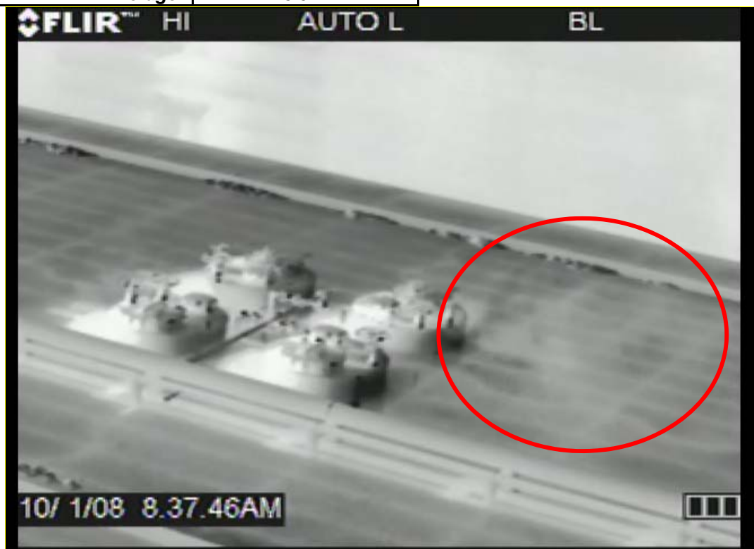
Figure G-4. Screenshot from FLIR Camera Showing Leak from 10/1/ 2008, Event #2
