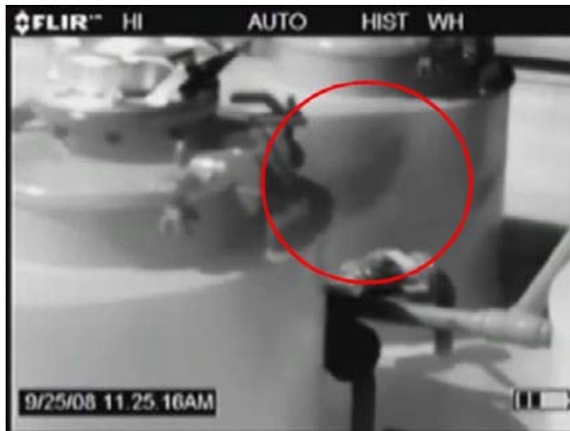
Figure 3-5. Leak from Cargo Hatch on Barge G2- Mass Leak 1.86 g/s
