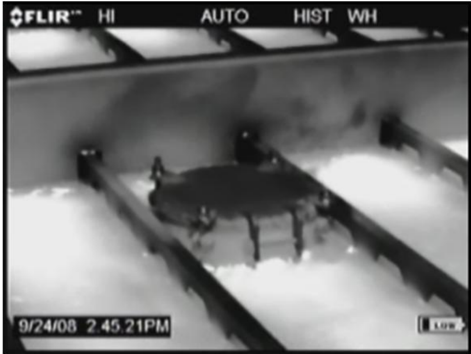
Figure D-5. Leak from Barge G1 (captured while onboard barge)
