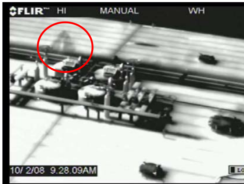
Figure 3-20. Example #3 from Ground Survey with LDEQ Camera – Leaking Valve from Barge L13- Total OTM 10 Mass Emission from Barge 0.106 g/s
