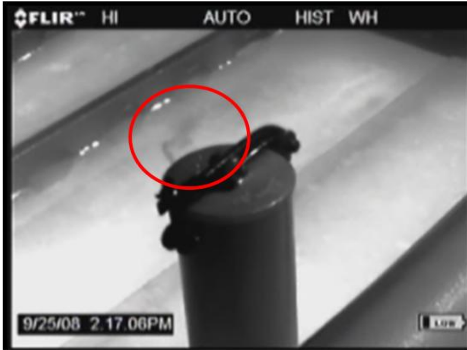
Figure D-15. Leak from Barge G3 (captured while onboard barge)
