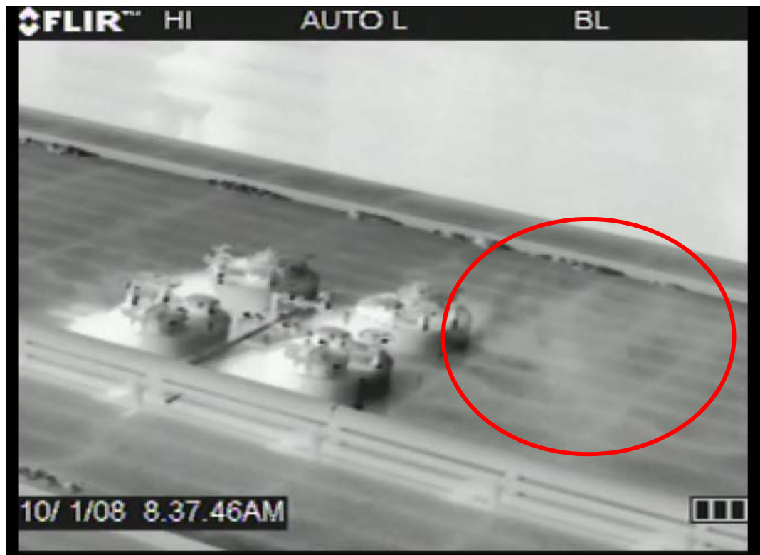
Figure 4-3. Screenshot from FLIR Camera Showing Leak from 10/1/ 2008, Event #2
