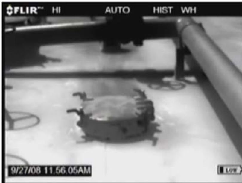
Figure 3-12. Leak from Cofferdam Hatch on Barge G6- Mass Leak 1.99 g/s
