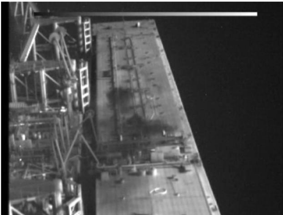
Figure B-14. Leak from Barge A32
