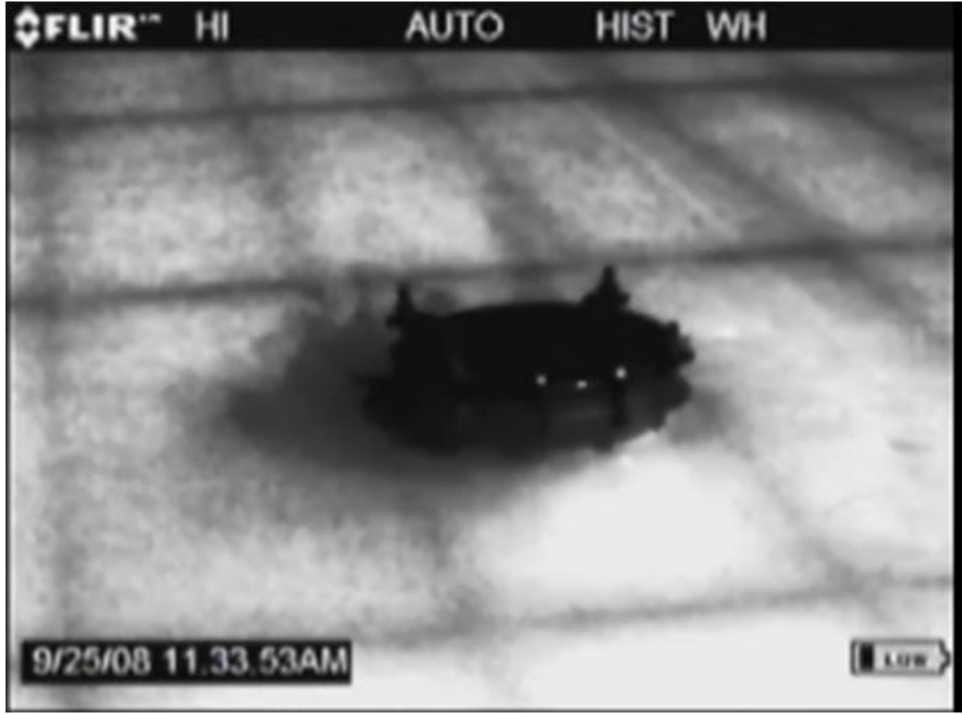
Figure D-10. Leak from Barge G2 (captured while onboard barge)
