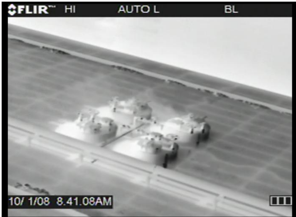
Figure E-5. Leak from Hatch 10/1
