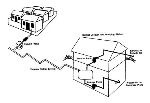
**Figure 5.2.** Typical vacuum sewer system schematic (Hassett 1995)
