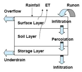
Figure 3-8. Conceptual diagram of a bio-retention cell LID.
