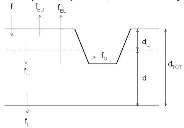
Figure 3-7. Two-zone groundwater model.
