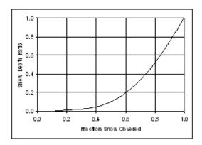
Figure 3-2. Areal Depletion curve for a natural area.
