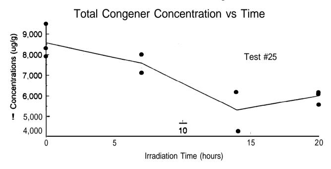
Figure 1. W Treatment of Gas Pipeline Soil
