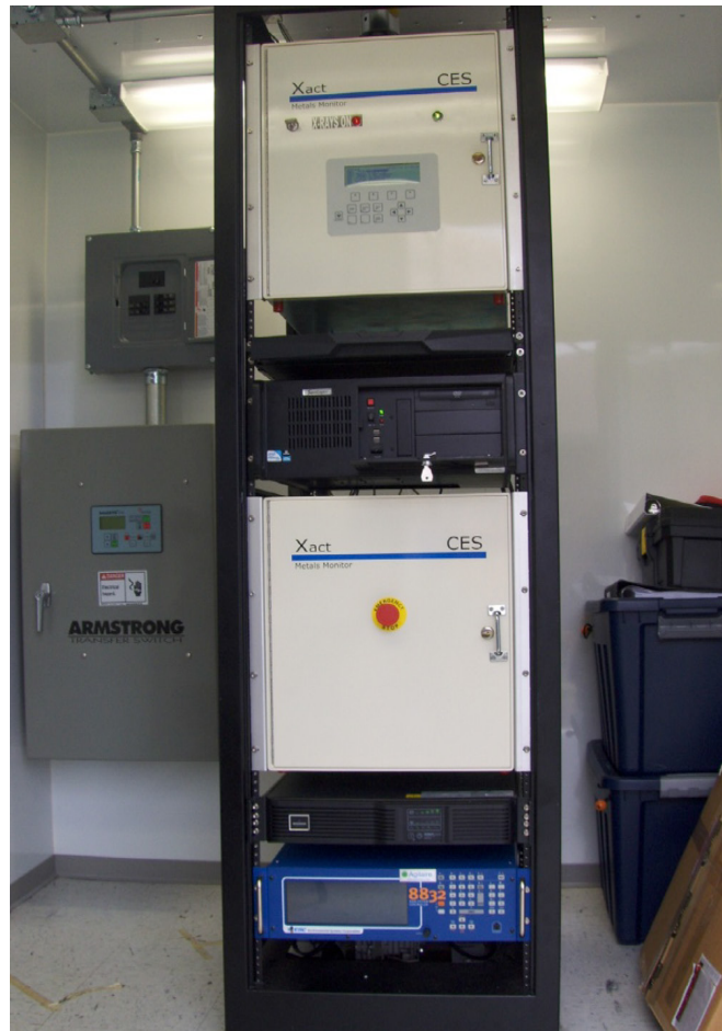
Figure 2-1. Xact 625 installed in field trailer for testing; top to bottom are the control panel/X-ray source, computer, XRF analysis module with sampling tape drive, modem, and datalogger.
