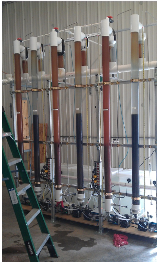
Figure 4. Pilot biological water treatment system for ammonia removal at the Iowa study site.
