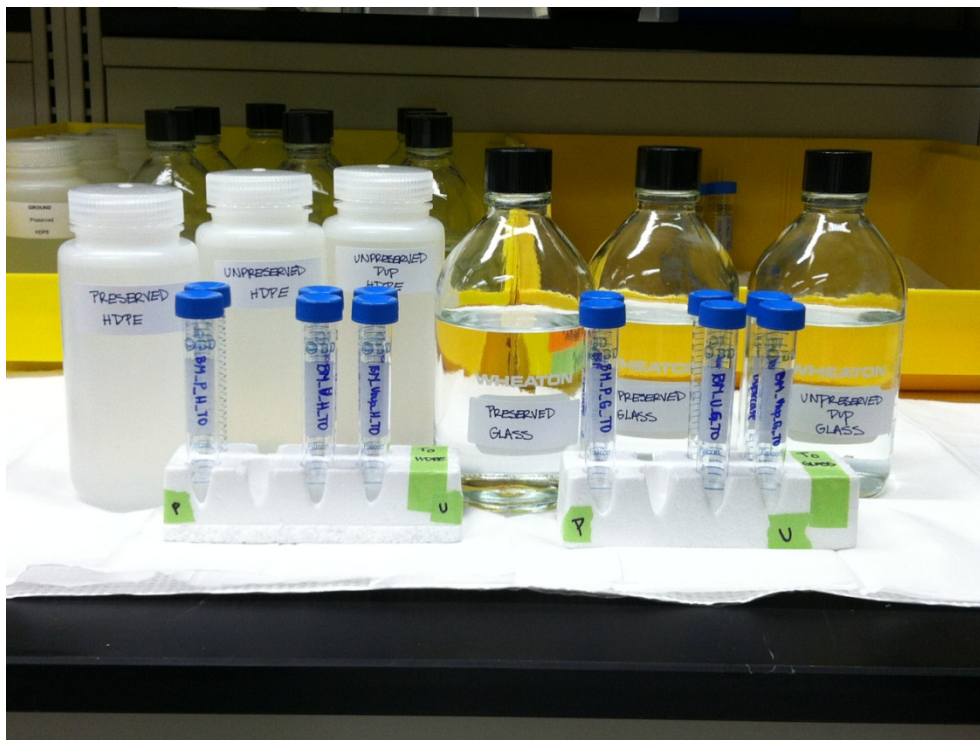
Figure 3. Duplicate 2 mL aliquots from each sample bottle (HDPE versus glass) were collected for lead analysis at specified time intervals in Phase One.
