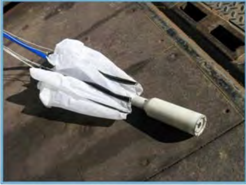
The Sahara Video sensor head and drogue.
