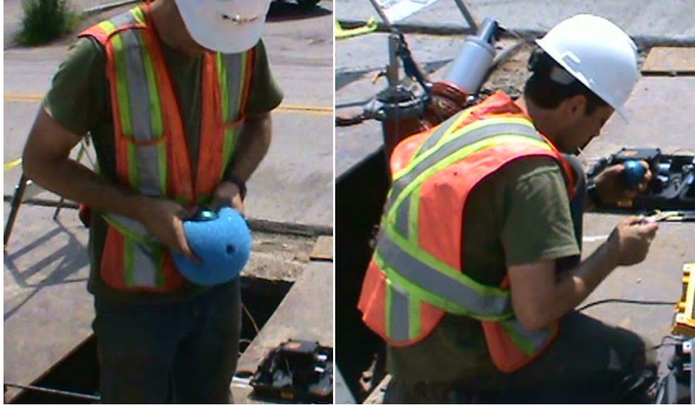
Figure 3-6. Aluminum Case and Foam Housing for SmartBall™ Acoustic Acquisition Device, Data Storage, and Power Supply
