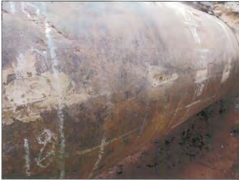
FIGURE 4.8 - EXTERNAL MACHINED DEFECTS
