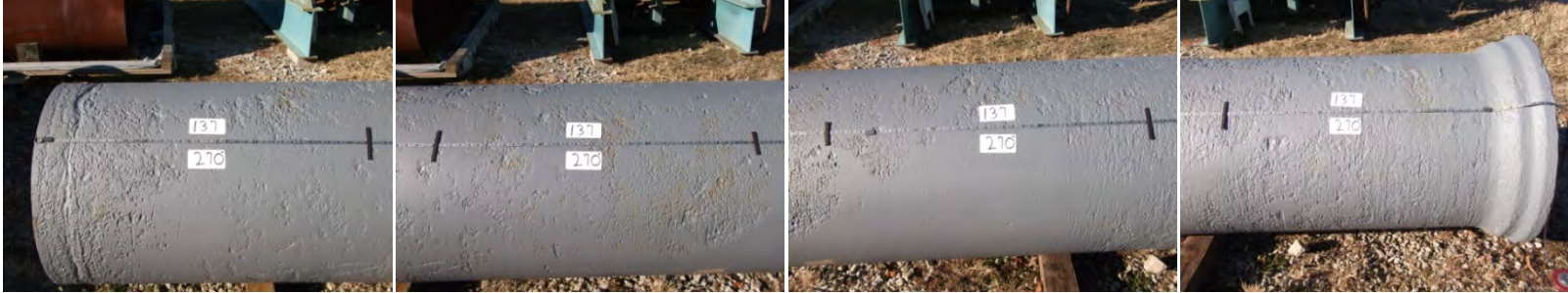
Figure A-137(2). Pipe 137 after Sandblasting
