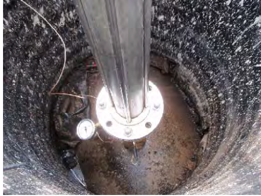
Figure 3-5. Accelerometer Acoustic Sensor Attached to the Sahara® Insertion Tube
