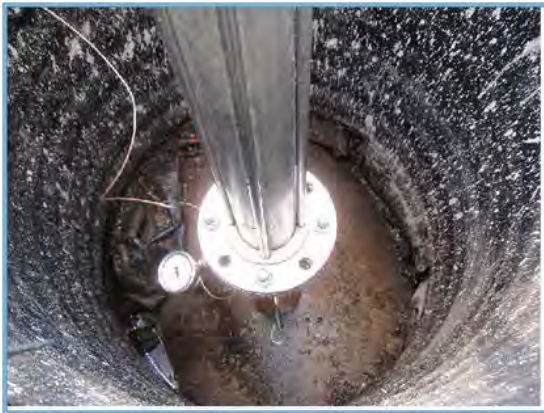
Accelerometer acoustic sensor attached to the Sahara insertion tube.
