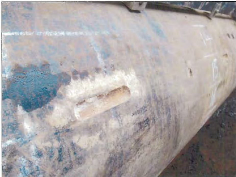
FIGURE A5.9 - PHOTOGRAPH OF MACHINED DEFECTS IN THE PIPE
