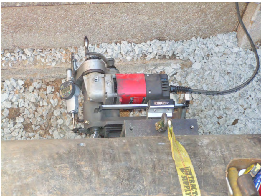
Figure 3-28. Magnetic Base End Mill Used to Create Machined Defects
