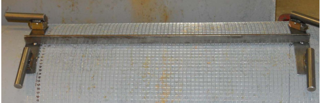
Figure 4-2. Bridging Bar Used to Establish a Reference for Measurements
