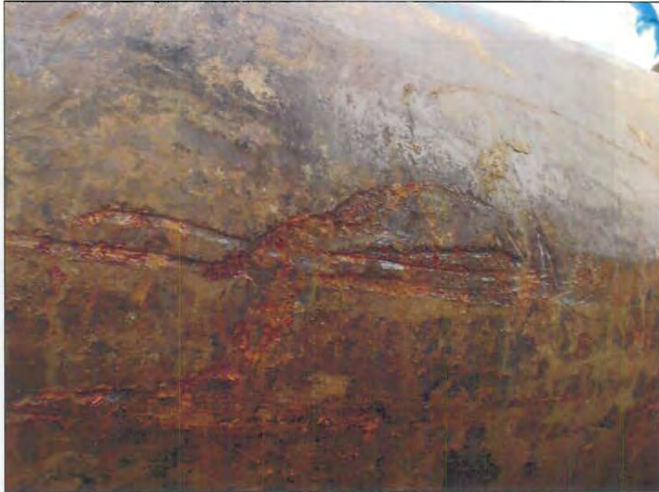
FIGURE A5.5 - PHOTOGRAPH OF MECHANICAL DAMAGE AND CORROSION
