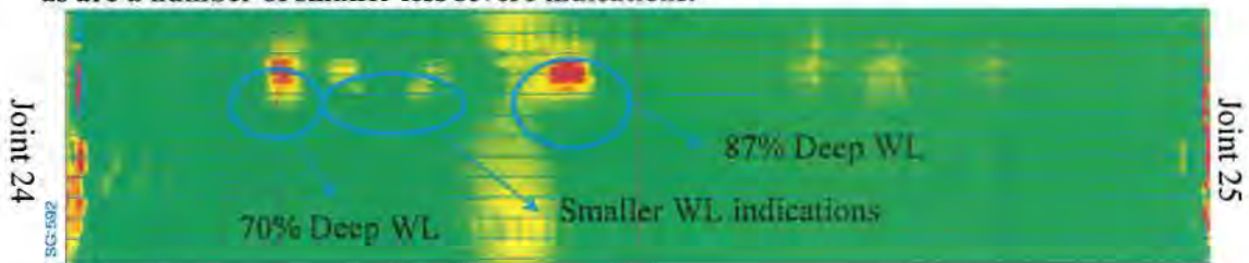
Figure 1. Colour map of See Snake RFT data for pipelength between joints 24 and 25. Red localized indications depict areas of substantial wall loss (WL).
