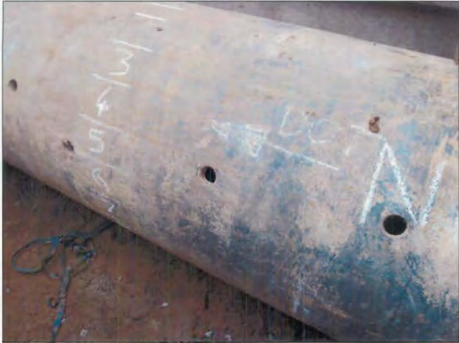
FIGURE A5.10 - PHOTOGRAPH OF MACHINED THREADED HOLES IN THE PIPE
