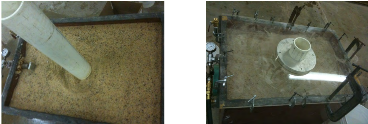
Figure 4-2. Top view of the chamber a) Filled with sand and b) Top closed using a Plexiglas plate.
