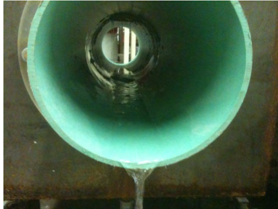
Figure 4-4. Typical I&I Flow Leak in the Test Model
