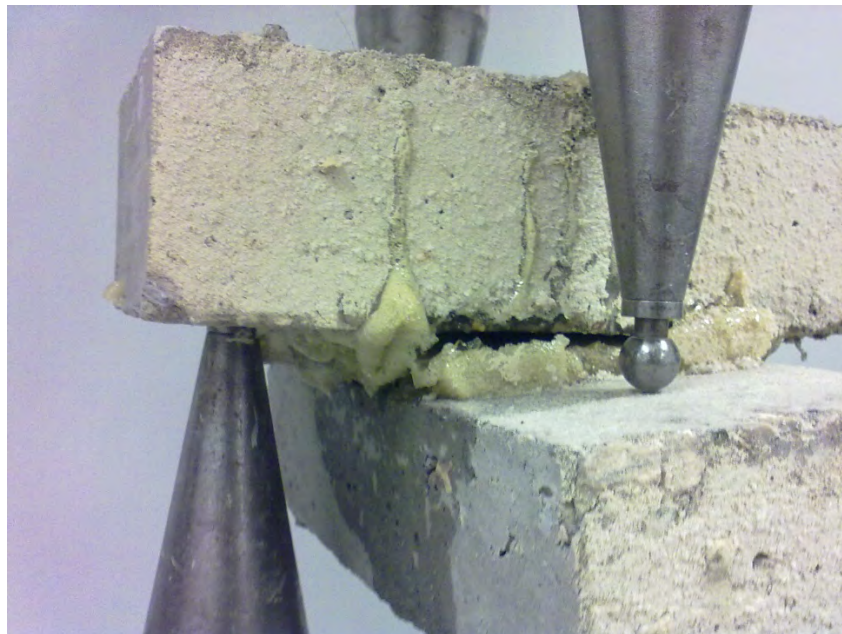
Figure 4.2. Typical failed specimen (Type 3 failure pattern).
