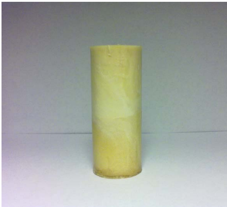
Figure 2-1. Polyurethane grout specimen (GST #3).
