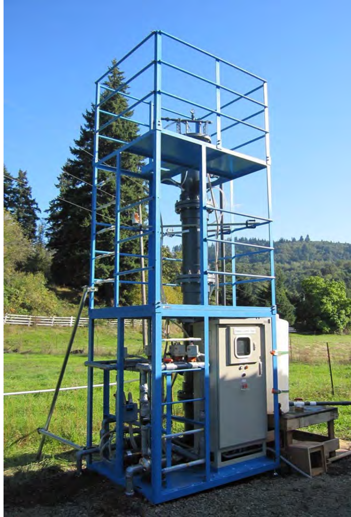
Figure 2-4. Photo of CHEMILES CLT-300 Pilot Unit at Test Site.
