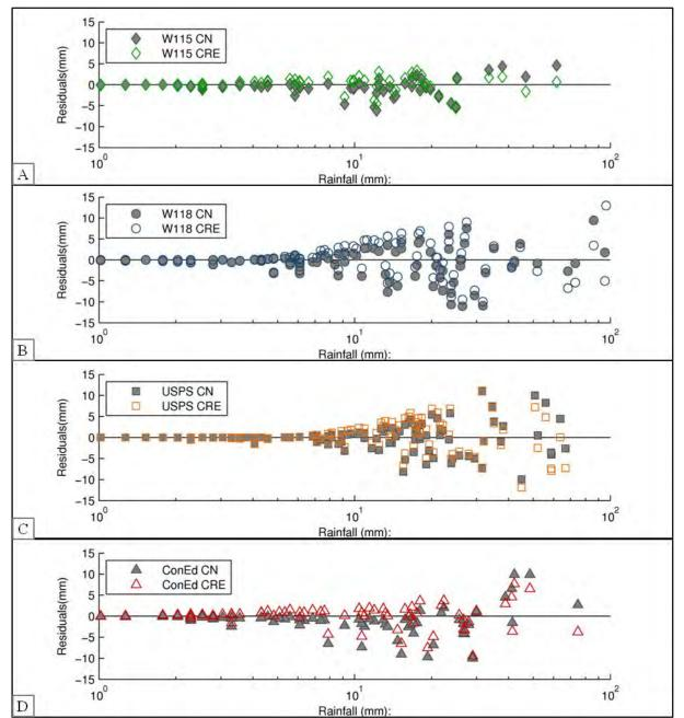
Figure 4-5: Residuals between characteristic runoff equations and curve number and observed depth for (A) W115, (B) W118, (C) USPS, and (D) ConEd.
