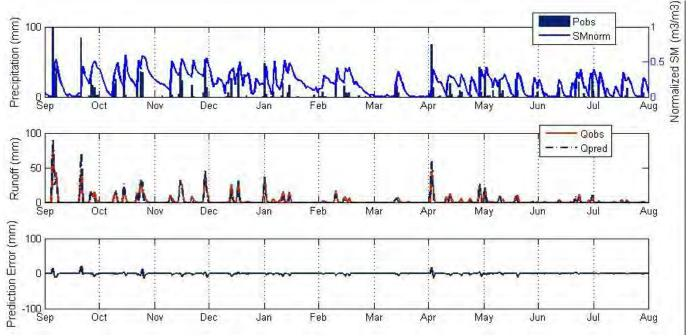
Figure 6-2 Precipitation, soil moisture, observed and simulated daily runoff and error for green roof W118.
