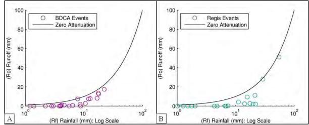
Figure 4-7: Characteristic runoff equations and events for (A) BDCA (B) Regis.
