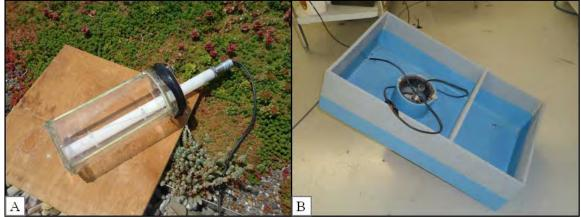
Figure 4-1: (A) Runoff monitoring weir device (B) Calibration chamber used to simulate rooftop runoff.
