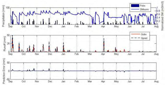
Figure 6-3: Precipitation, soil moisture, observed and simulated daily runoff and error for green roof W115.
