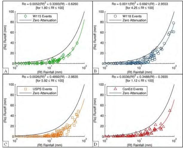
Figure 4-4: Characteristic runoff equations and events for (A) W115, (B) W118, (C) USPS, and (D) ConEd.
