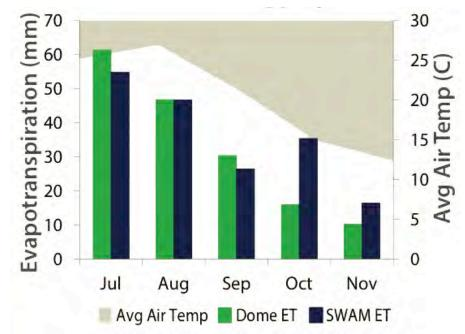
Figure 6-5: Comparison of measured versus modeled evapotranspiration (Dome ET to SWAM ET) on W118.
