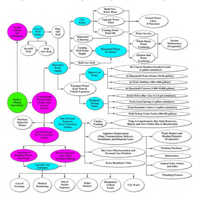
Figure 2.1 - Flow chart of the impacts of mining contaminants on drinking water
