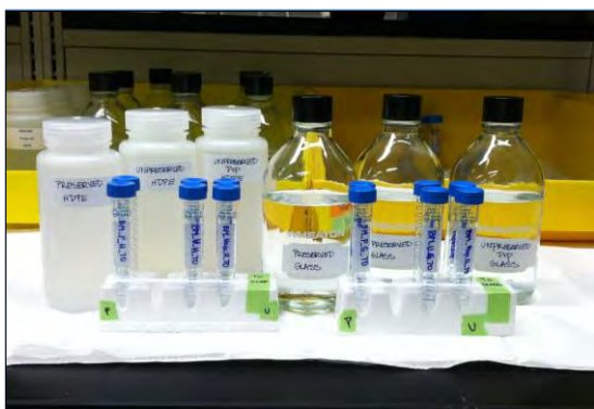
Figure 2. LEFT: Duplicate 2 mL aliquots from each sample bottle (HDPE versus glass) were collected for lead analysis at specified time intervals in Phase One. RIGHT: Representative results of lead concentration in DI water contained in glass and HDPE bottles in Phase 1.
