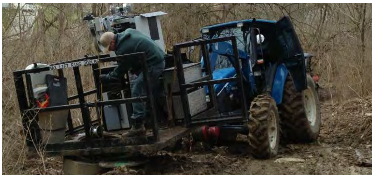
Figure 1-1. Custom Off-road CCTV Camera Tractor (Courtesy: MSDGC)
