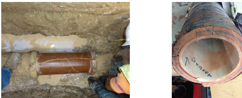
Figure C-16. Denver Irving St.: Images of the HDPE Liner Section during Retrieval (left) and in the TTC Laboratory (right)
