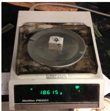
Figure A-4. Weight Measured in Air (left) and in Water (right)
