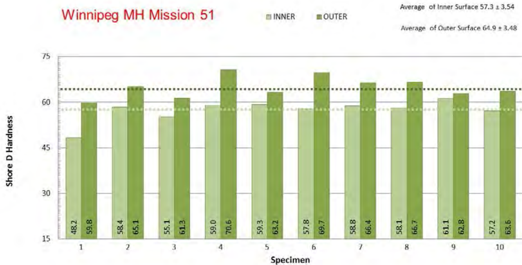
Figure B-100. Winnipeg 3: Shore D Hardness Readings from Inner and Outer Surfaces
