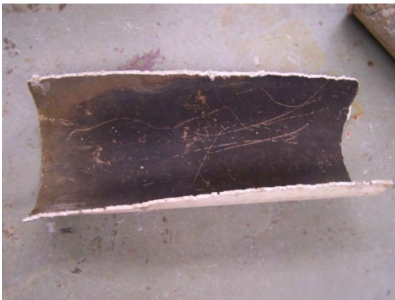
Figure B-68. New York 2: Images of the Inner Surface of the 23-Year Old, 36-in. Long CIPP Liner Section Prior to Testing
