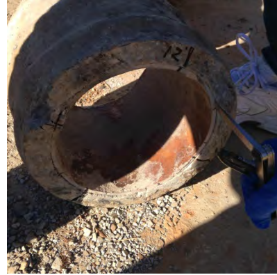
Figure B-52. Nashville 1: Retrieval of the Sample (left) and Measuring Annular Gap on the Received Sample (right)
