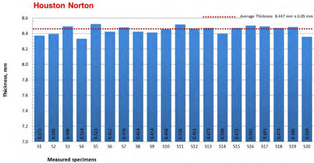
Figure C-52. Houston-Norton Dr.: Average Thickness of the Liner Sample
