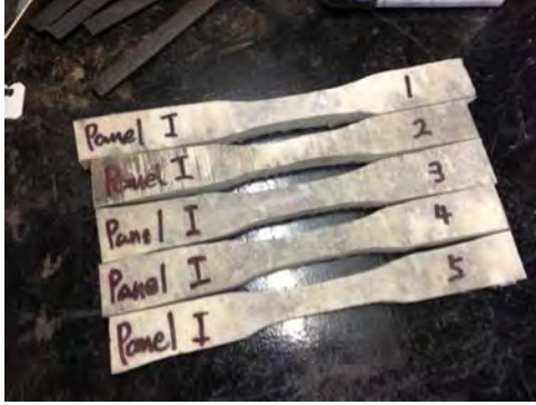
Figure B-44. Indianapolis: Five Panel 1 Specimens (left) and Five Panel 2 Specimens (right) Prepared for Tensile Testing
