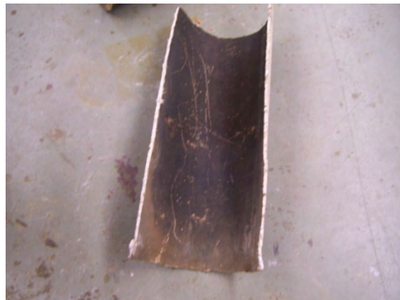
Figure B-68. New York 2: Images of the Inner Surface of the 23-Year Old, 36-in. Long CIPP Liner Section Prior to Testing
