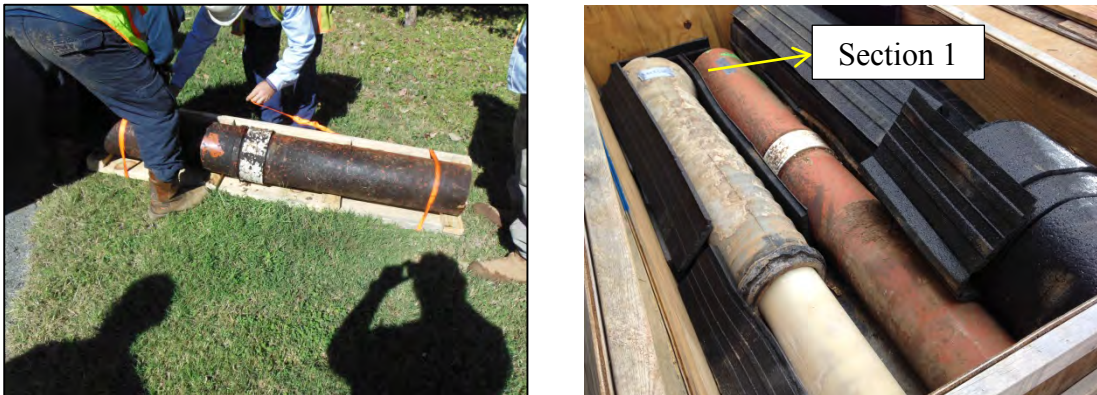
Figure C-9. Nashville Elaine Dr.: Images of the PVC Liner Section after Retrieval (left) and Samples Received at the TTC Lab (right)
