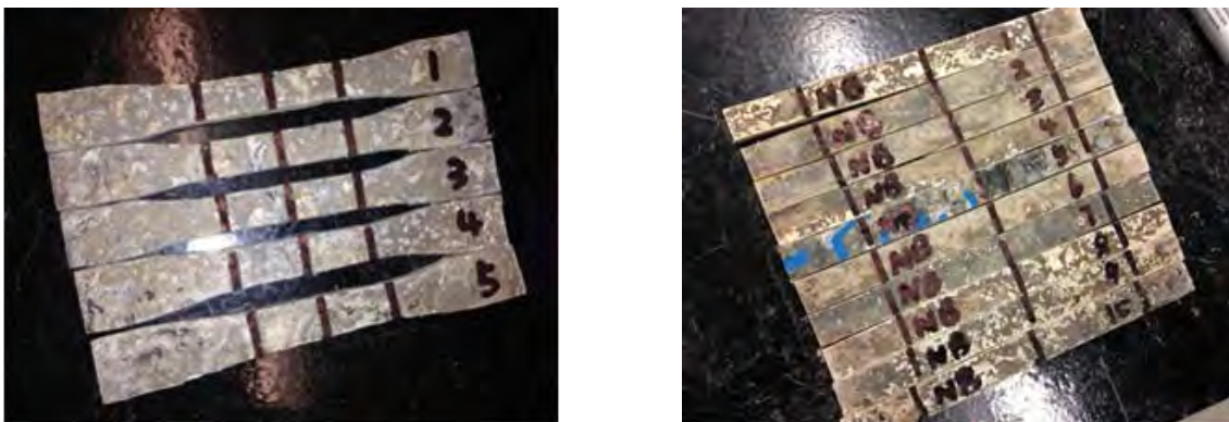
Figure A-2. ASTM D638 Specimens (left) and ASTM D790 Specimens (right)
