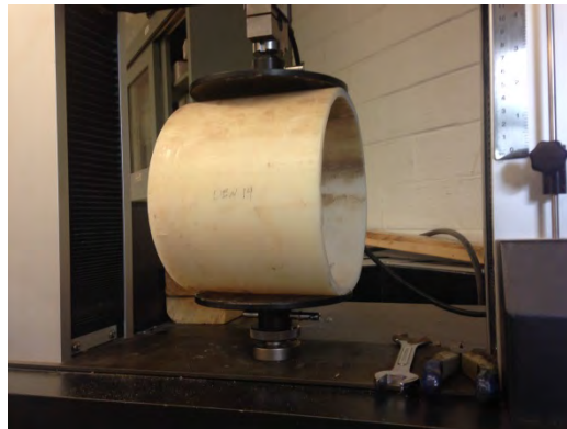
Figure C-8. Denver Rigsby Ct.: Parallel Plate Test
