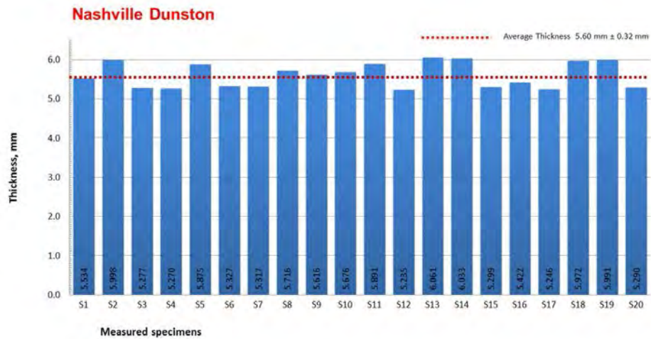
Figure B-54. Nashville 1: Average Thickness of the Sample
