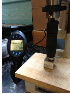
Figure A-5. Hardness Test Instrument (left) and Hardness Test on a Specimen (right)
