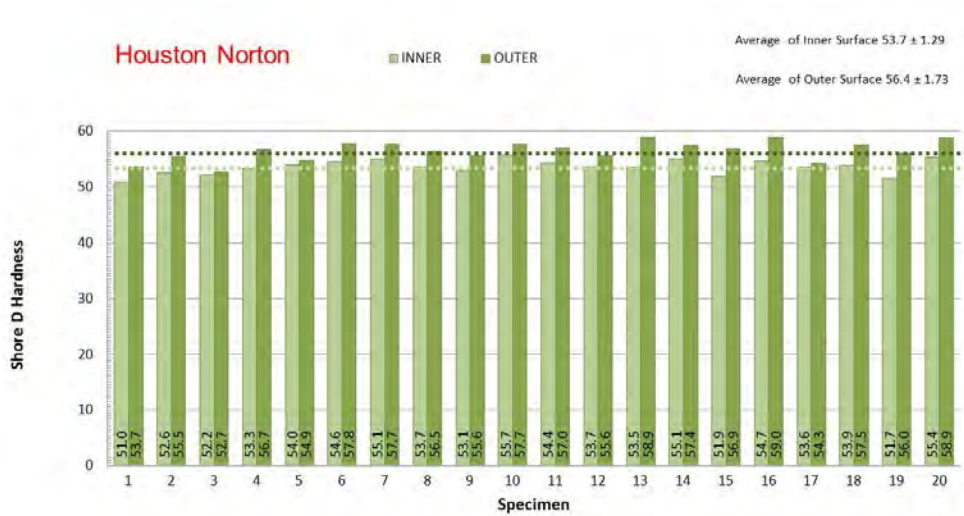
Figure C-56. Houston Norton Dr.: Shore D Hardness Readings for the Liner’s Inner and Outer Surfaces
