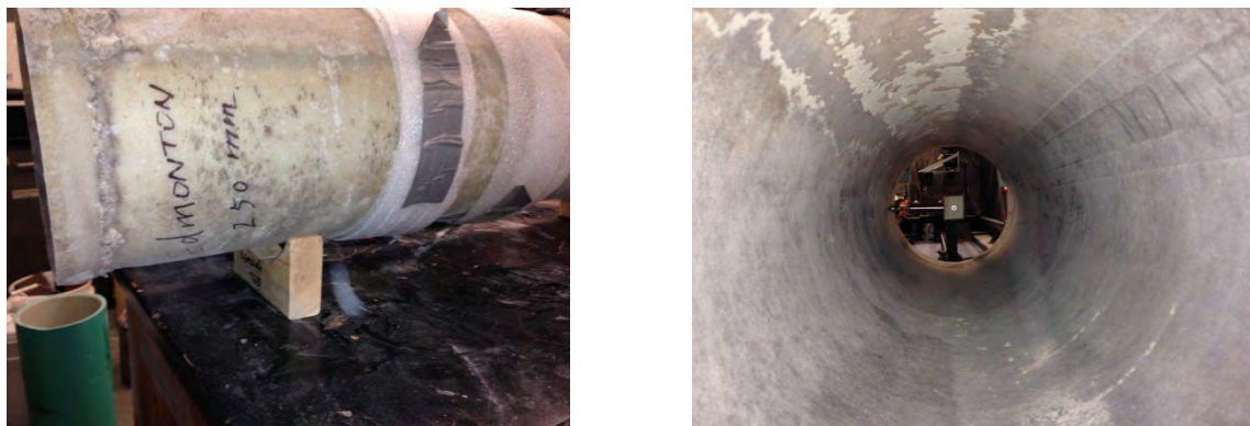
Figure B-3. Profile Plotter Setup (left) and Ovality Measurement (right)
