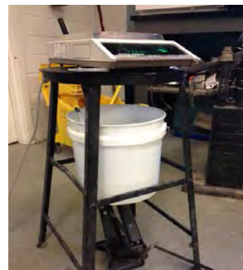
Figure A-4. Weight Measured in Air (left) and in Water (right)
