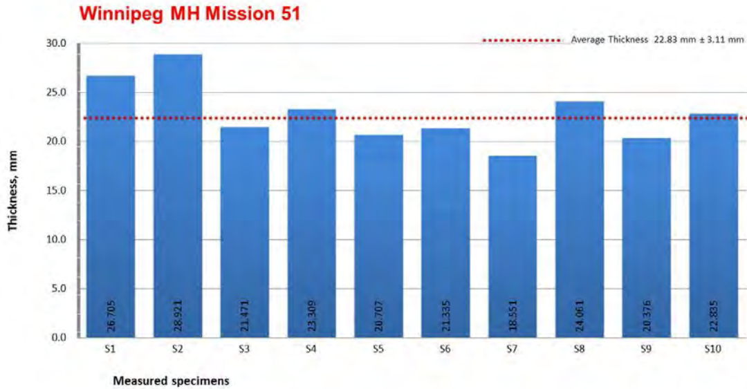
Figure B-98. Winnipeg 3: Average Thickness of the Sample
