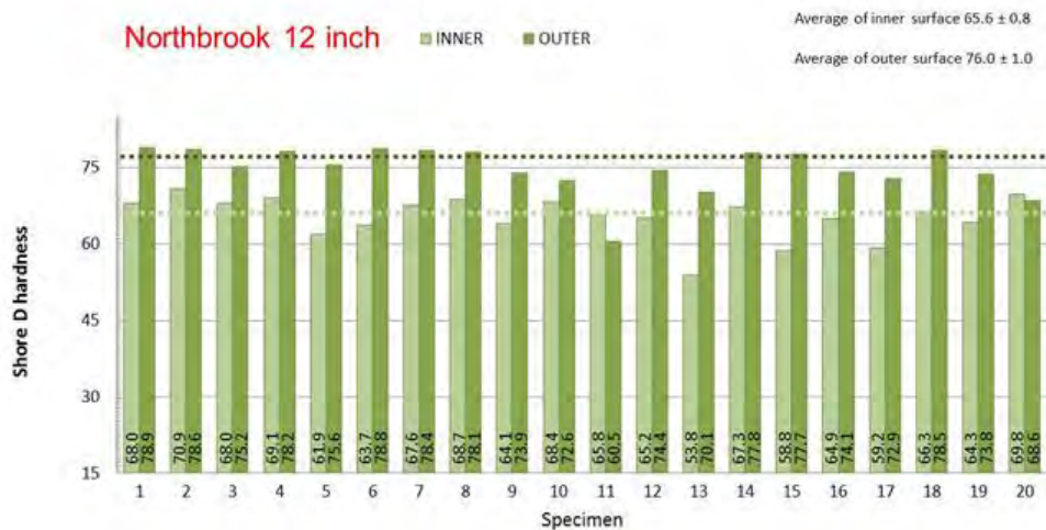
Figure B-87. Northbrook: Shore D Hardness Readings from Inner and Outer Surfaces
