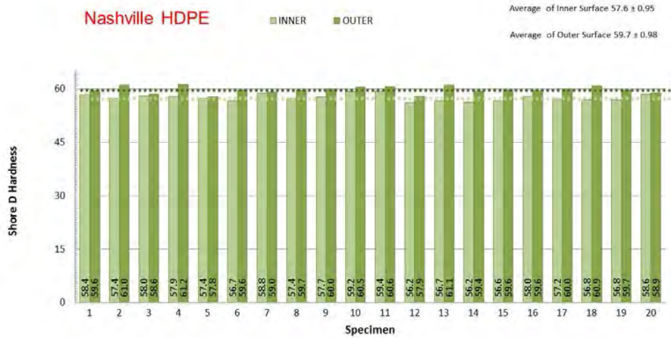
Figure C-40. Nashville Danby Dr.: Shore D Hardness Readings for the Liner’s Inner and Outer Surfaces
