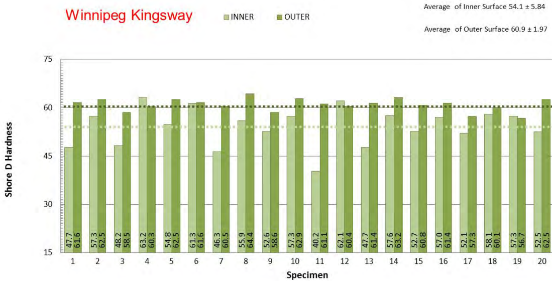
Figure B-96. Winnipeg 2: Shore D Hardness Readings from Inner and Outer Surfaces
