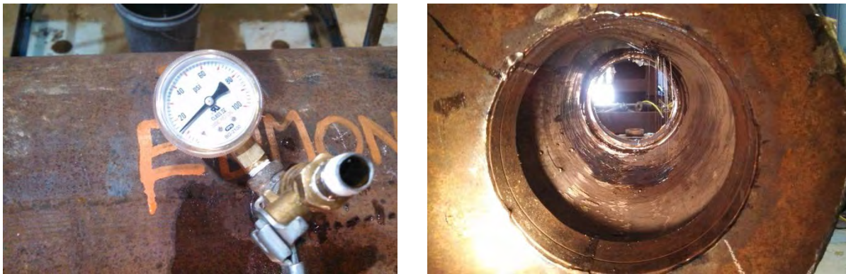
Figure B-14. Edmonton 1: Short-Term Buckling Test Setup
