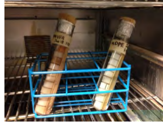
Figure C-41. Igepal CO-630 Reagent (left) and Specimens inside the Oven (right)
