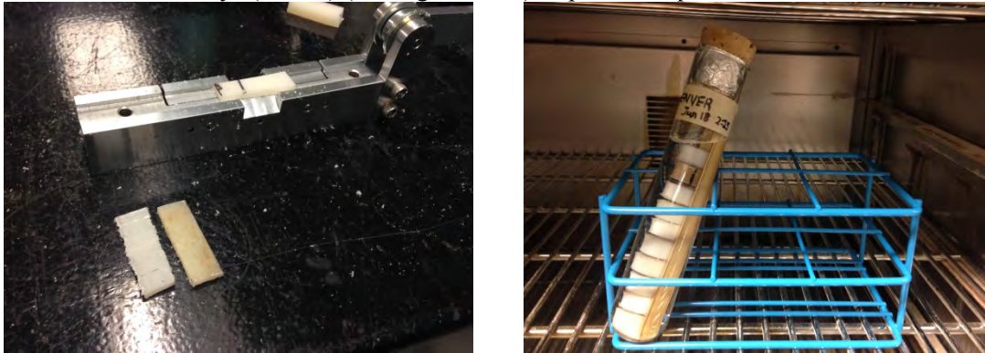
Figure C-23. Preparation of Test Specimen (left) and Specimens Inside the Oven (right)
