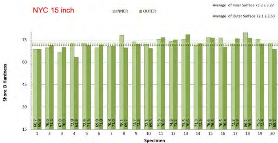
Figure B-73. New York 2: Shore D Hardness Readings for the Liner’s Inner and Outer Surfaces
