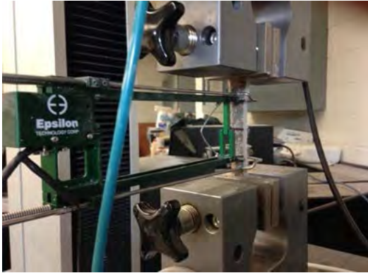
Figure A-3. ASTM D638 Test (left) and ASTM D790 Test (right)
