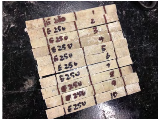
Figure B-10. Five Specimens (left) and 10 More Specimens (right) for Flexural Testing
