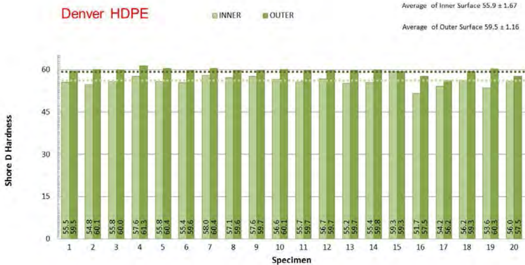
Figure C-22. Denver Irving St.: Shore D Hardness Readings for the Liner’s Inner and Outer Surfaces
