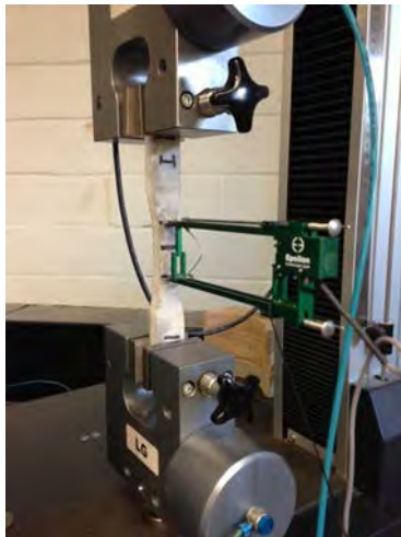
Figure B-45. Indianapolis: Tensile Testing in Accordance with ASTM D638 (left) and Samples after Test (right)
