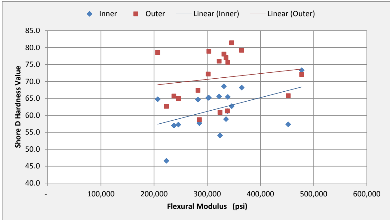
Figure 5-10. Shore D Hardness versus Flexural Modulus
