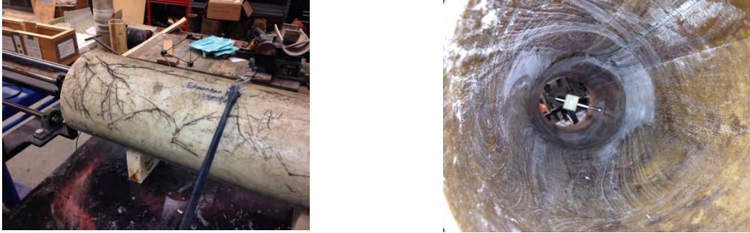
Figure B-16. Edmonton 2: Profile Plotter Setup (left) and Measurement of Ovality (right)
