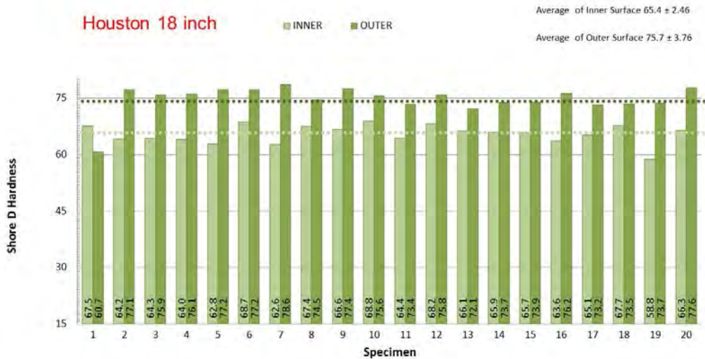
Figure B-37. Houston 2: Shore D Hardness Readings from Inner and Outer Surfaces
