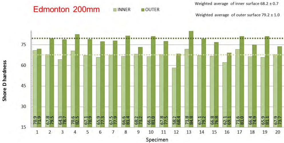
Figure B-22. Edmonton 2: Shore D Hardness Readings from Inner and Outer Surfaces
