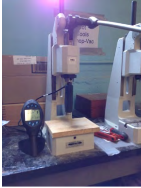
Figure A-5. Hardness Test Instrument (left) and Hardness Test on a Specimen (right)
