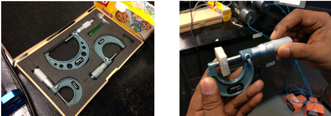
Figure A-1. Micrometer Set (left) and Measurement of Thickness Using a Micrometer (right)
