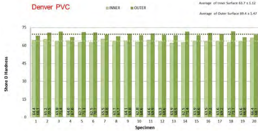
Figure C-7. Denver Ringsby Ct.: Shore D Hardness Readings for the Liner’s Inner and Outer Surfaces
