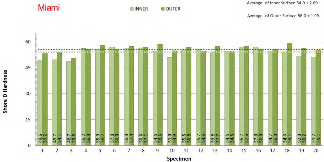
Figure C-31. Miami 114th St.: Shore D Hardness Readings for the Liner’s Inner and Outer Surfaces
