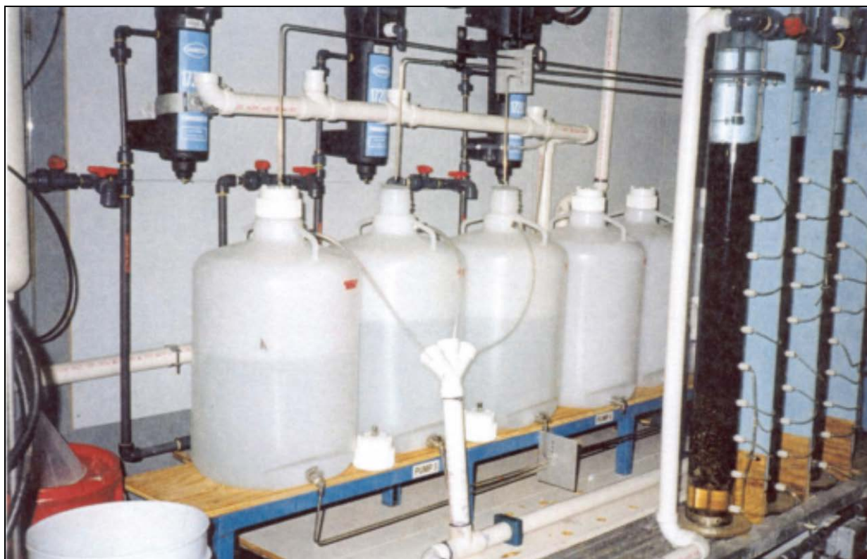
Figure B19a. Filtrate clearwells showing lines leading to waste and to backwash.
