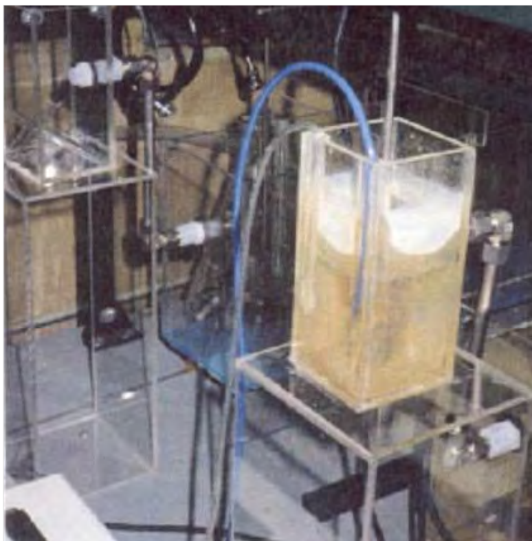
Figure B5. Rapid mixing chamber with influent and alum feed lines.
