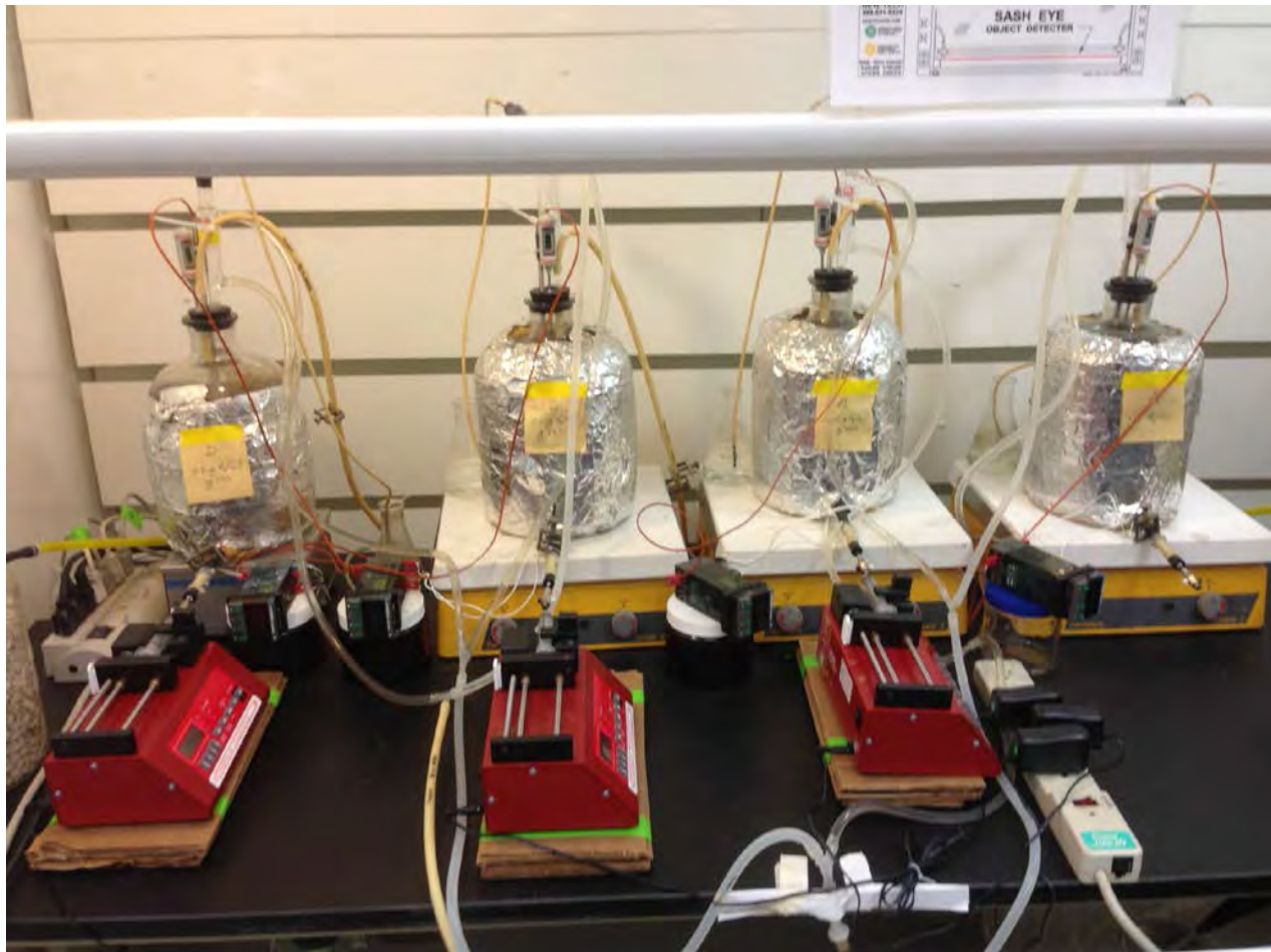
Figure 3.1 Photograph of Aerobic Sludge Thermo-Oxidation Experimental System
