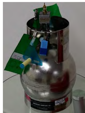
Figure 13. Active air sampling canister (SUMA canister).
