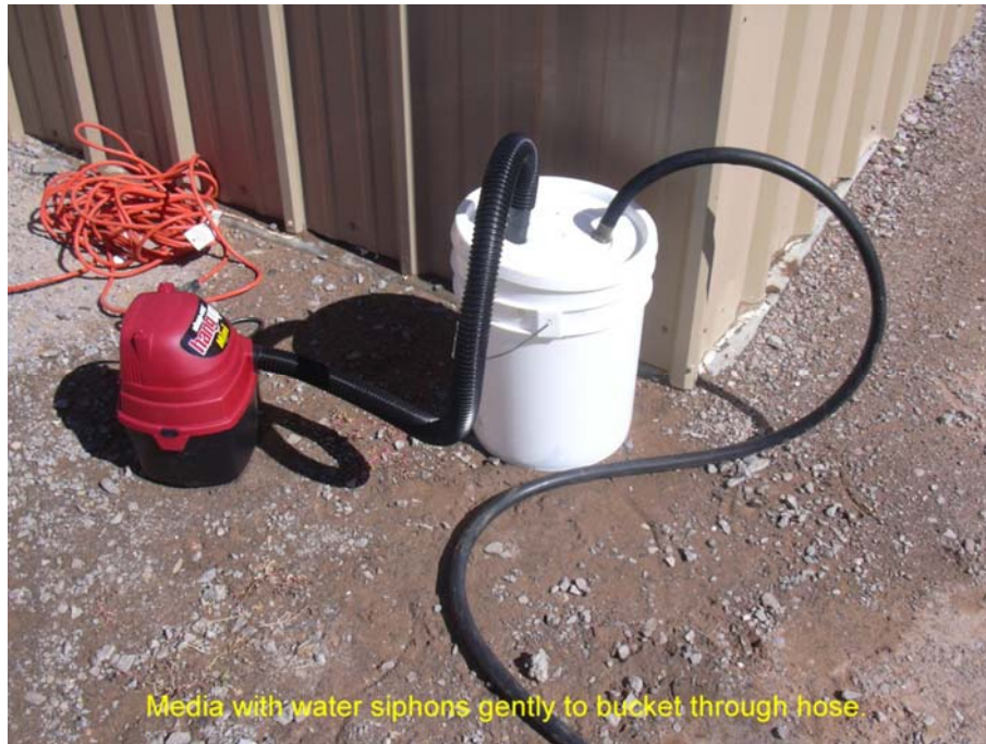
Figure 3-2. Apparatus Used for Spent Media Sampling
