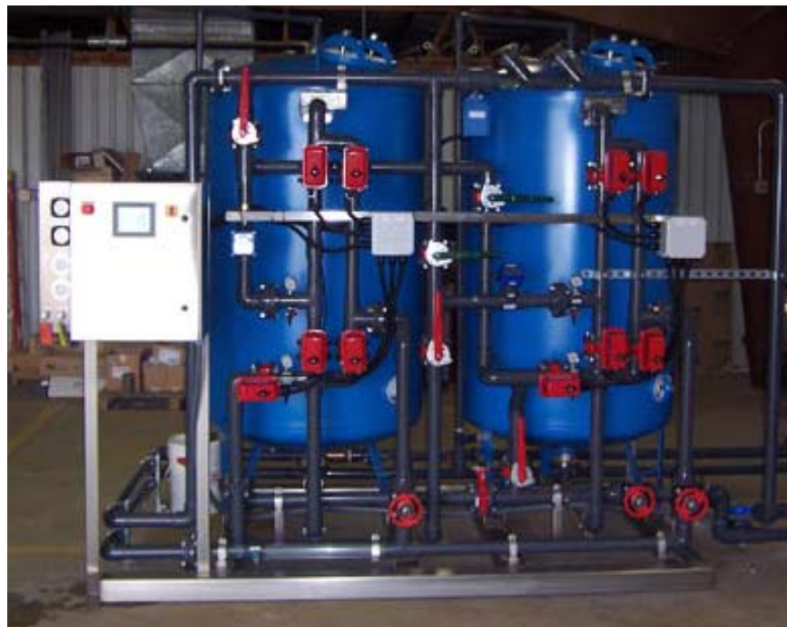
Figure 4-9. Adsorption System Valve Tree and Piping Configuration
