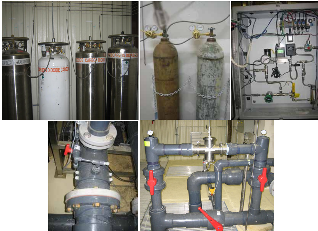
Figure 4-12. Carbon Dioxide Gas Flow Control System for pH Adjustment (Clockwise from Top Left: CO 2 Supply Assembly with Four 380-lb Dewars and Two 50-lb Cylinders; pH Control Panel; Sanitary Cross and CO 2 Loop; and Port for pH Probe)
