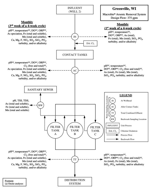
Figure 2. Process Flow Diagram and Sampling Schedules
