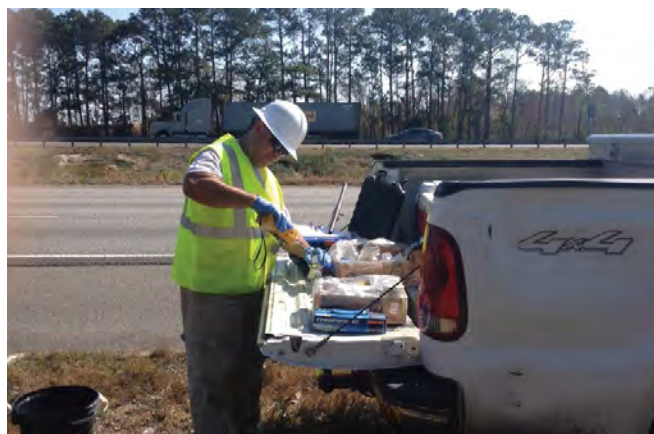
At the scene of a diesel spill on a highway in Jacksonville, Florida, Ruben Rodriguez is testing a soil sample, using a glass jar and a photoionization detector.
