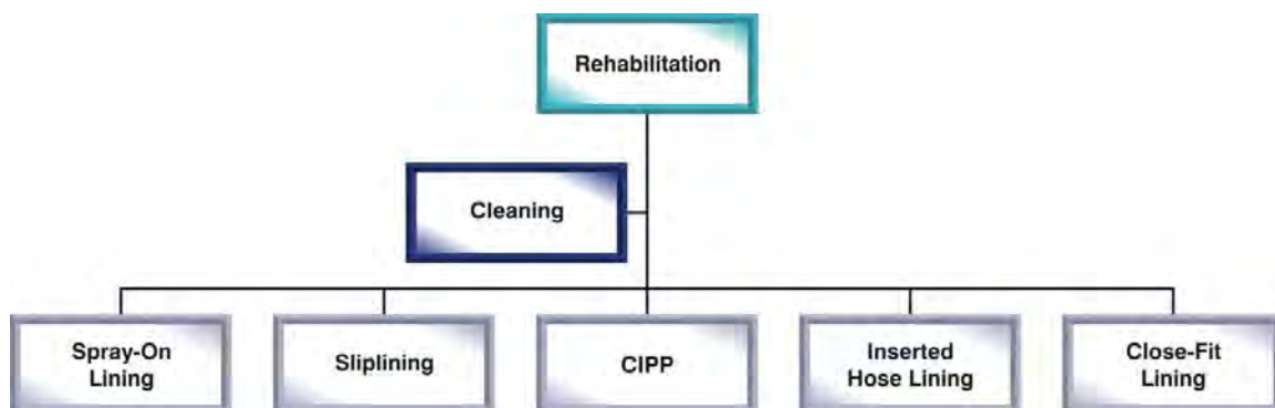
Figure 3-2. Rehabilitation Approaches for Water Mains (EPA, 2013)
