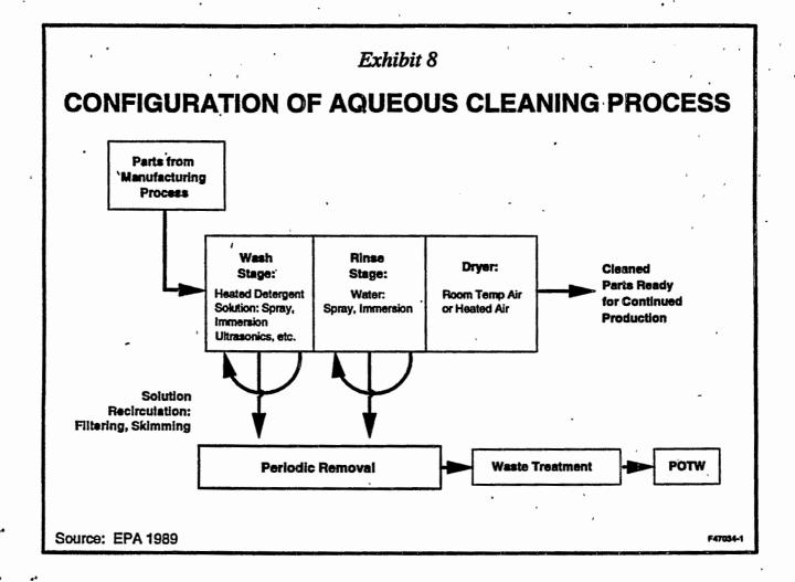
as a source of air. Blowers are capable of removing 90 percent or more of water from parts. Design options in blowers include variation of pressure, velocity, and volume flow. Other sources of air include dedicated compressors and plant air. Plants should use filters to remove oil, particles, and moisture to achieve the desired level of air quality. When using the forced air drying method, issues such as noise, humidity, and air conditioning may have to be considered.
