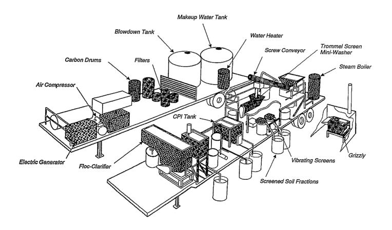
Figure A-1. Typical VRU Operational Setup.
