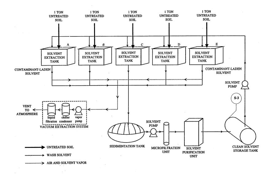
Figure 1-1. Schematic diagram of the Terra-Kleen technology.
