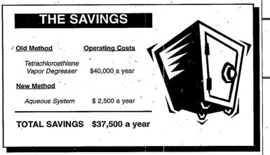
solids removed from the bottom of the machines. This disposal cost is approximately \$2,000 per year for all four machines. Thus, Inland Steel has replaced purchases and disposal costs of \$40,000 per year associated with tetrachloroethylene with costs of approximately \$2,500 per year for aqueous cleaning (see Exhibit 7).
