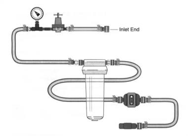
Be sure that the filter housing does *not* contain the filter.
