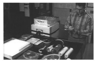
Each month, your laboratory will send you all of the equipment needed to collect samples for *Giardia* cyst and *Cryptosporidium* oocyst analyses. When you receive the sampling kit, check the contents of the carton. The sampling kit should contain the following items:
