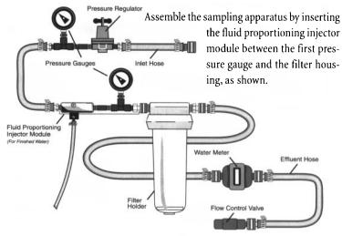
Connect the inlet end of the sampling apparatus to the sampling tap or to an extension hose connected to the tap.
