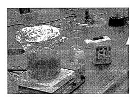
Remove the electrode from the beaker, and pour the contents of the beaker into a centrifuge bottle.
