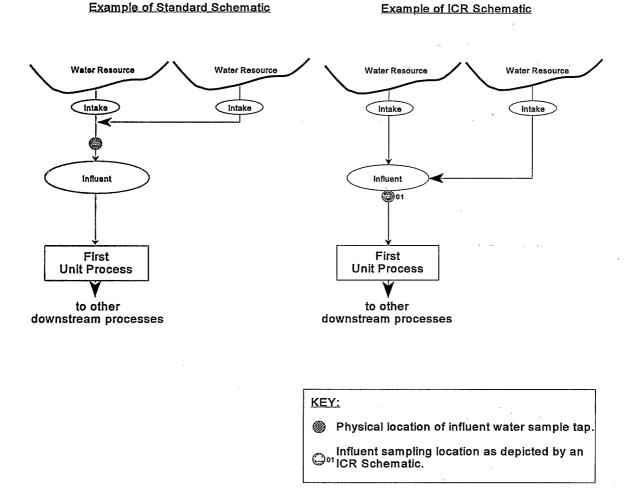
Figure 5-2. Treatment Plant Influent Sample - Multiple Intakes
