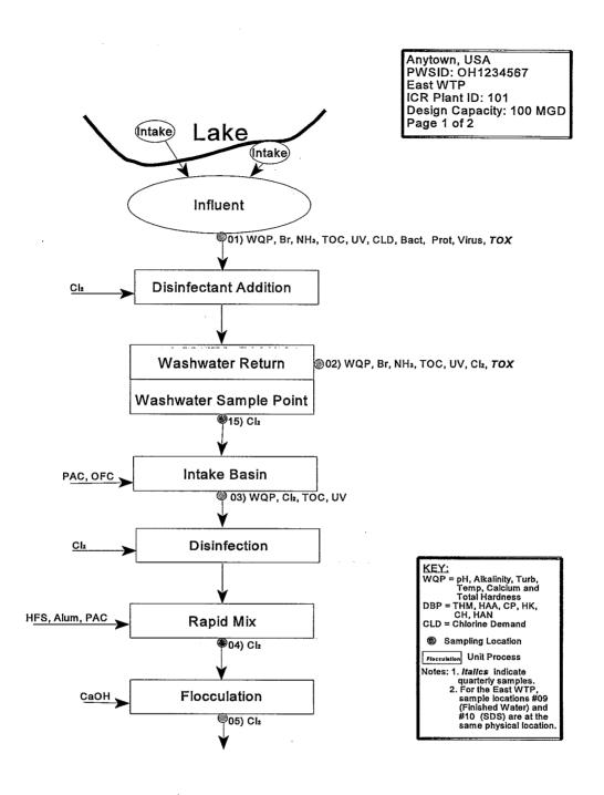
Figure 2-1. ICR Water Treatment Plant Schematic (Example)
