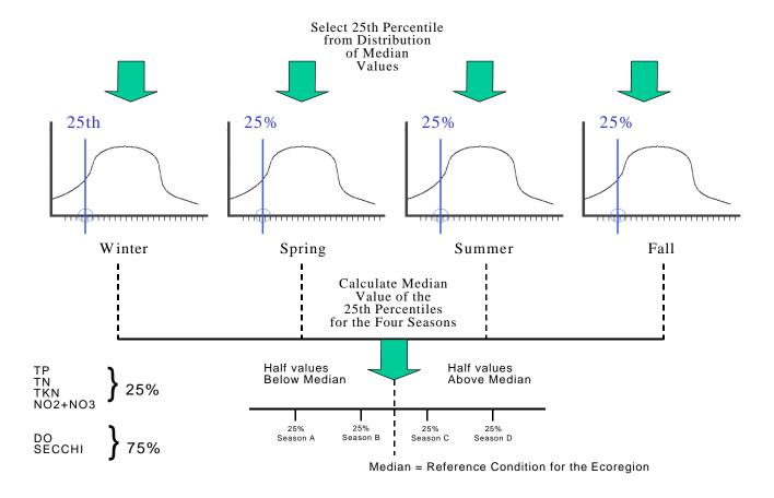
Figure 4b. Illustration of reference condition calculation.
