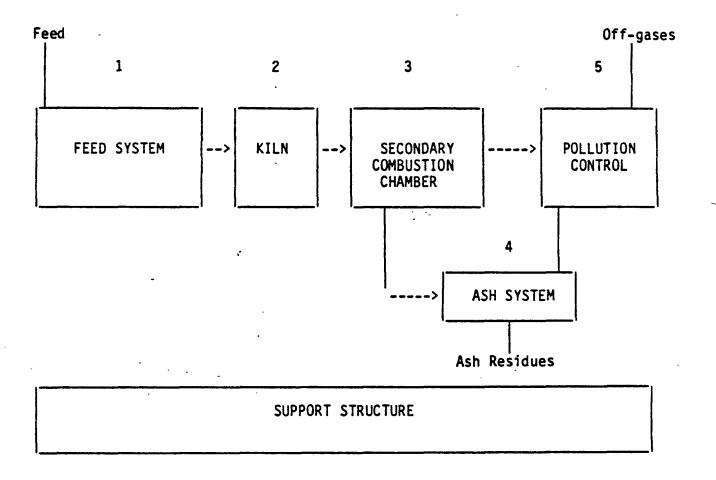
Figure 1. Mobile Incinerator Components
