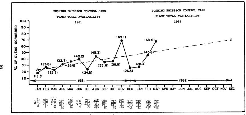
Figure 6. Availability of all operating H-III systems (combined) at U.S. Steel/Clairton (supplied by U.S. Steel).
