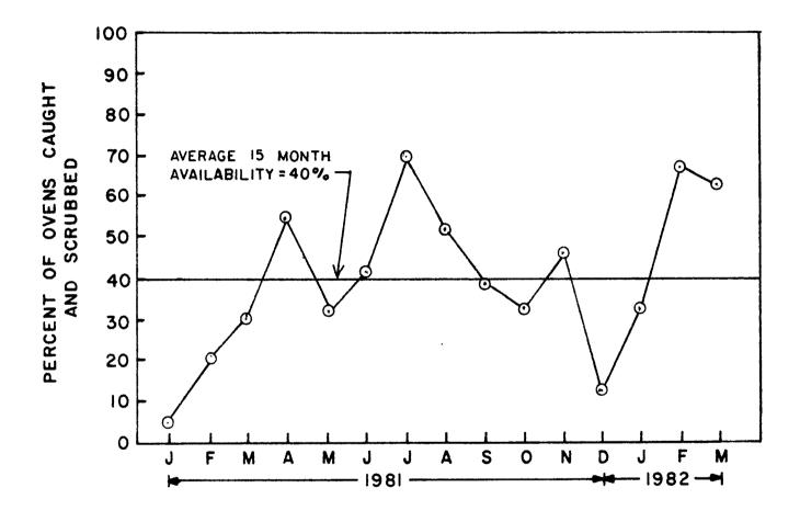
Figure 4. Availability data for H-III serving Batteries 19 and 20 at U.S. Steel/Clairton.
