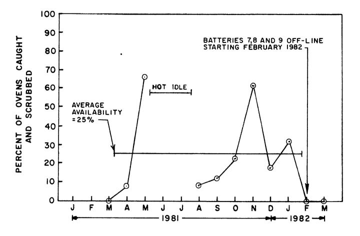
Figure 2. Availability data for H-III serving Batteries 7, 8 and 9 at U.S. Steel/Clairton.
