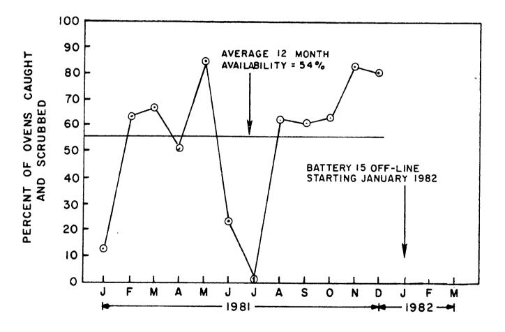
Figure 3. Availability data for H-III serving Battery 15 at U.S. Steel/Clairton.
