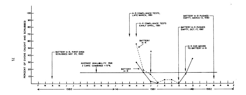
Figure 8. Availability data for H-III at J&L/Indiana Harbor Works (two cars, two batteries). Additional data not available from EPA or J&L.
