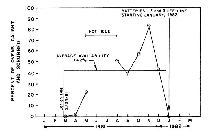
Figure 1. Availability data for H-III serving Batteries 1, 2 and 3 at U.S. Steel/Clairton. Average shown for 7 months operation, March 1981 through December 1981, excluding hot idle downtime.
