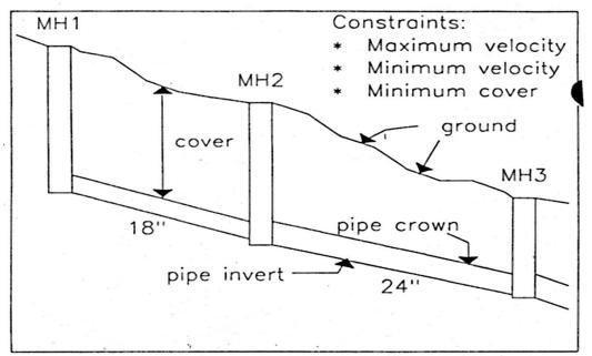
Figure 2-1. Profile view of the vertical alignment of a stormwater system (Miles and Heaney, 1988) (Reproduced with permission of the American Society of Civil Engineers).
