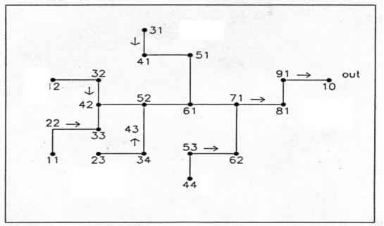
Figure 2-2. Layout of the twenty pipe stormwater problem (Miles and Heaney, 1988) (Reproduced with permission of the American Society of Civil Engineers).
