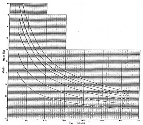
Figure 5-4. Intensity-duration-frequency curves for Boulder, CO (From US SCS, 1973).
