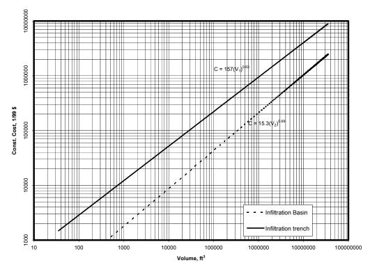
Note: V<sub>1</sub>= trench volume; V<sub>2</sub>=basin volume Figure 4-4. Construction cost, infiltration trenchs and basins (Adapted from Young et al., 1996).
