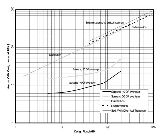
Note: OF = overflow Figure 4-5. Operation and maintenance costs for CSO controls (Adapted from US EPA 1993).
