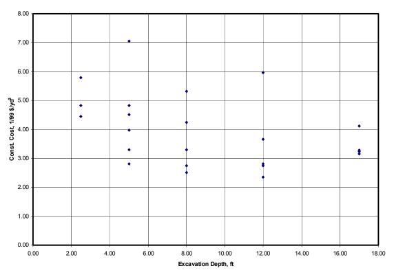
Figure 3-2. Trench excavation costs (Updated from RS Means, 1996a).
