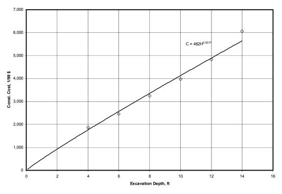
Figure 3-3. Manhole costs, as a function of excavation depth.
