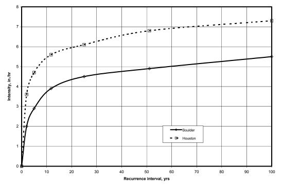
Figure 5-6. Intensities vs. recurrence interval for Boulder, CO and Houston, TX for a 20-min duration.
