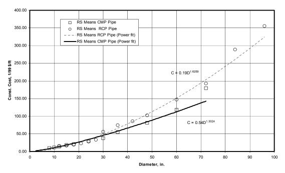
Figure 3-1. Cost of storm drainage pipe.
