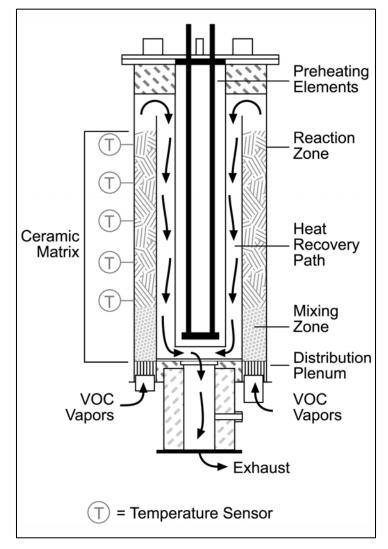
Figure 3-2. Flameless Thermal Oxidizer System
