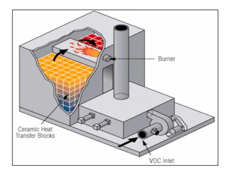
Figure 3-5. Regenerative Thermal Oxidizer
