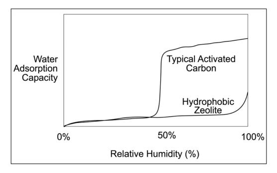
Figure 4-4. Comparison of Humidity Effects on Adsorption Capacity of Adsorbents
