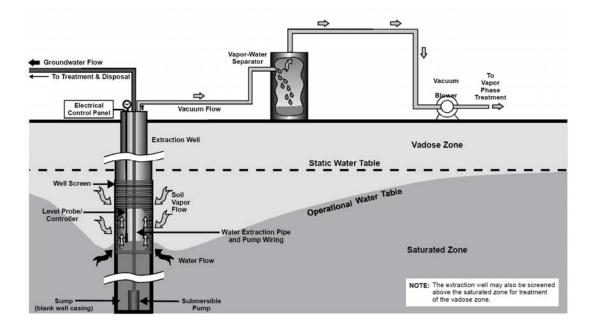
Figure 2-2. Typical Multi-Phase Extraction System
