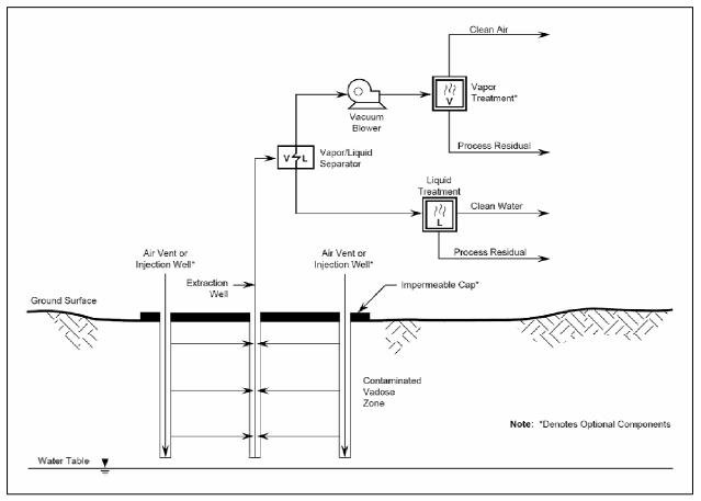
Figure 2-1. Typical Soil Vapor Extraction System
